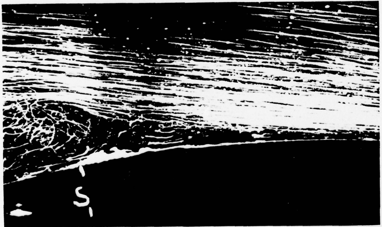
Fig. 5.3 Flow visualization of an upstream moving separation with R_e \sim 10^5
