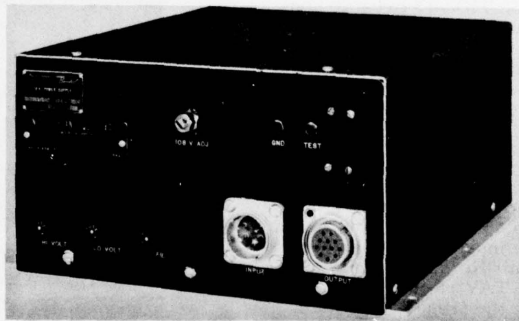
Figure A-10. Power supply unit No. 12. The power supply is a Bendix type TPP-7 dynamotor type unit capable of providing power for the entire telemeter transmitter. The input power requirement is 550 watts at 26 volts.
