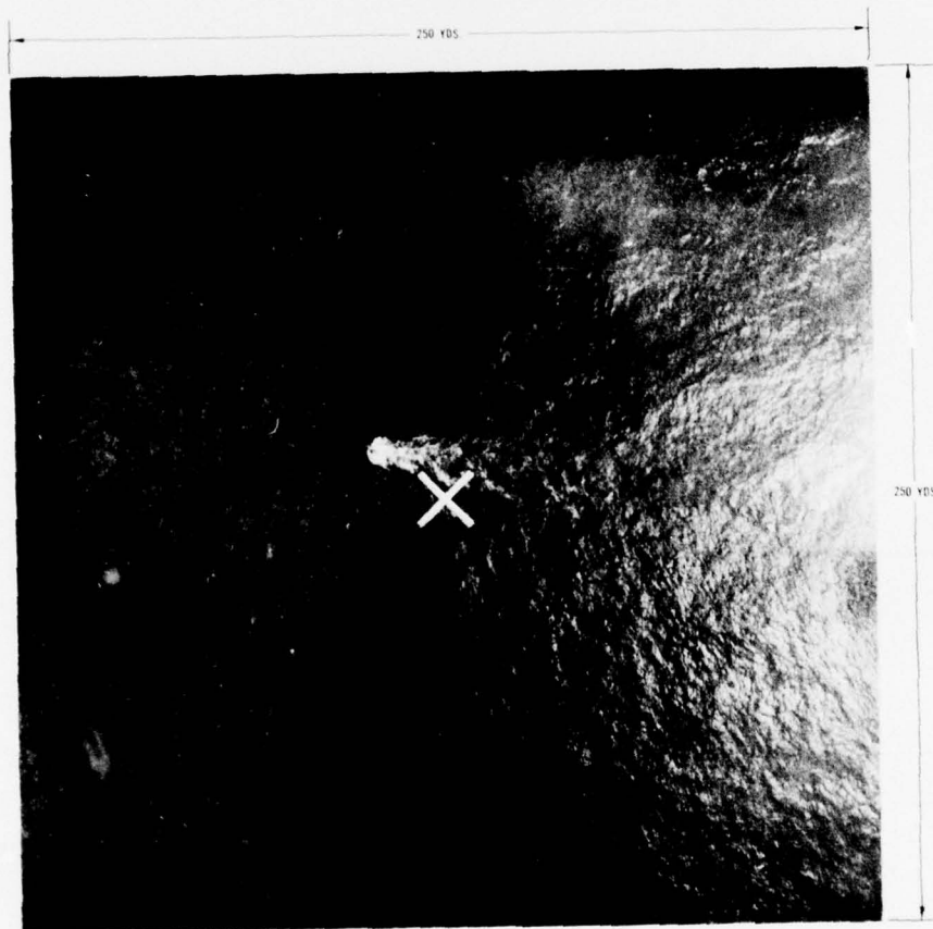
Figure 3. Vertical view of the sea surface taken from a helicopter at an altitude of 500 feet; the submarine's periscope is almost directly under the helicopter (indicated by cross).
