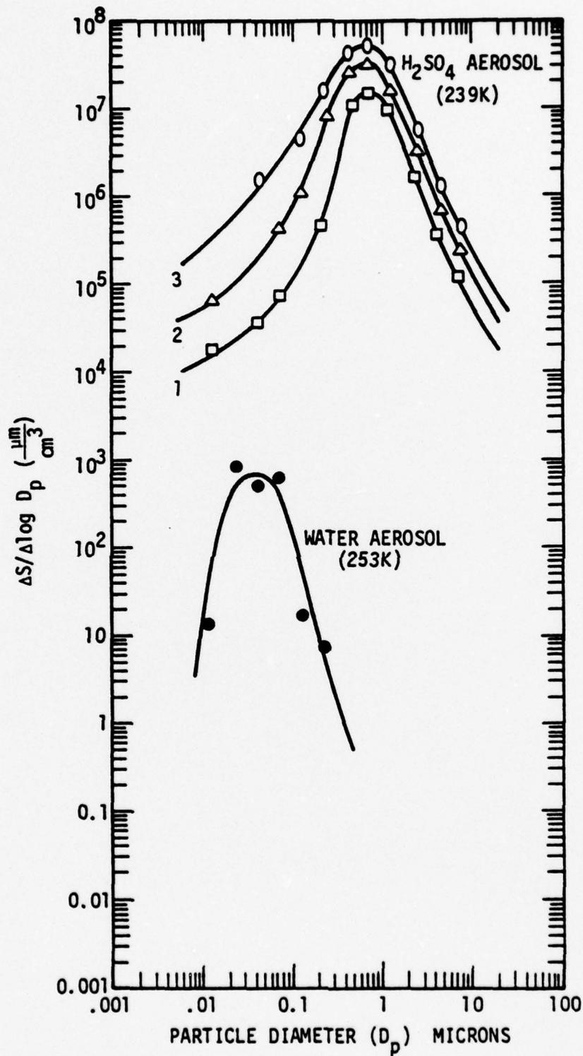
Figure 5. Log-normal Plot of Surface Area Concentration of  $\text{H}_2\text{O}$  and  $\text{H}_2\text{SO}_4$  Aerosols Generated in Flow Experiments. The Experimental Conditions are given in Table 1 & 2.
