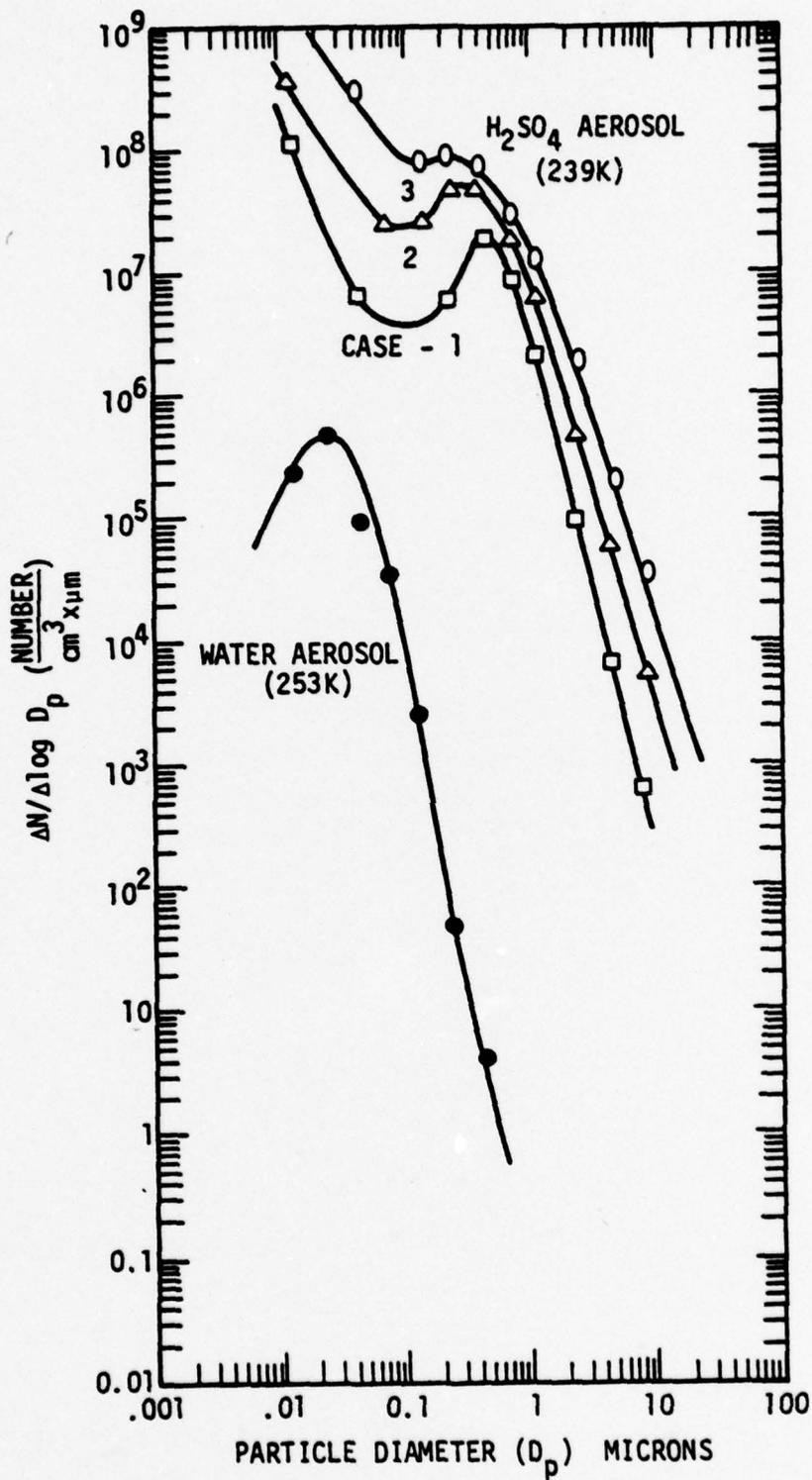
Figure 4. Log-normal Plot of Number Concentration of H<sub>2</sub>O and H<sub>2</sub>SO<sub>4</sub> Aerosols Generated in Flow Experiments. The Experimental Conditions are Given in Tables 1 & 2.
