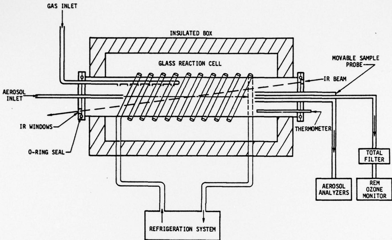
Figure 1. Schematic Diagram of Refrigerated Reaction Chamber
