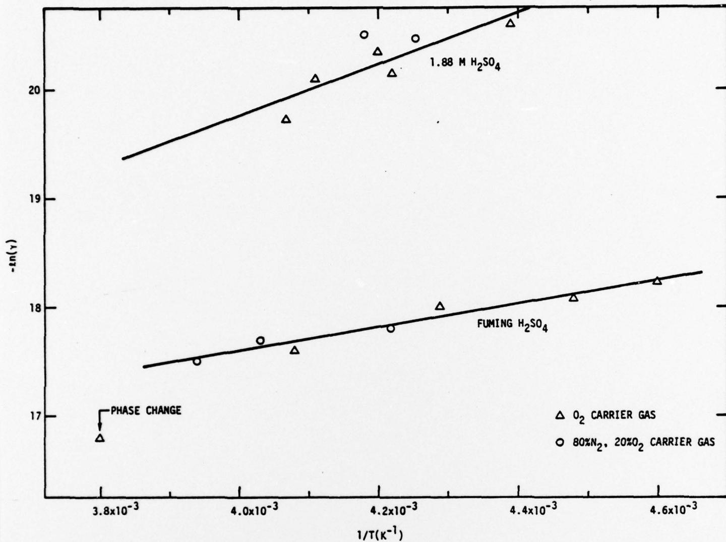
Figure 7. Semi-logarithmic Plot of the Measured Reaction Efficiency (reactions / collision) of the Ozone Decomposition Versus Reciprocal Absolute Temperature for Fuming  $H_2SO_4$  and Dilute  $H_2SO_4$  in  $H_2O$ .
