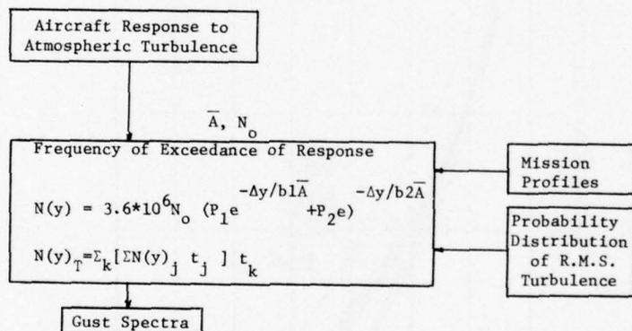
Fig.3.4.5.1 Basic approach to fatigue gust load determination
