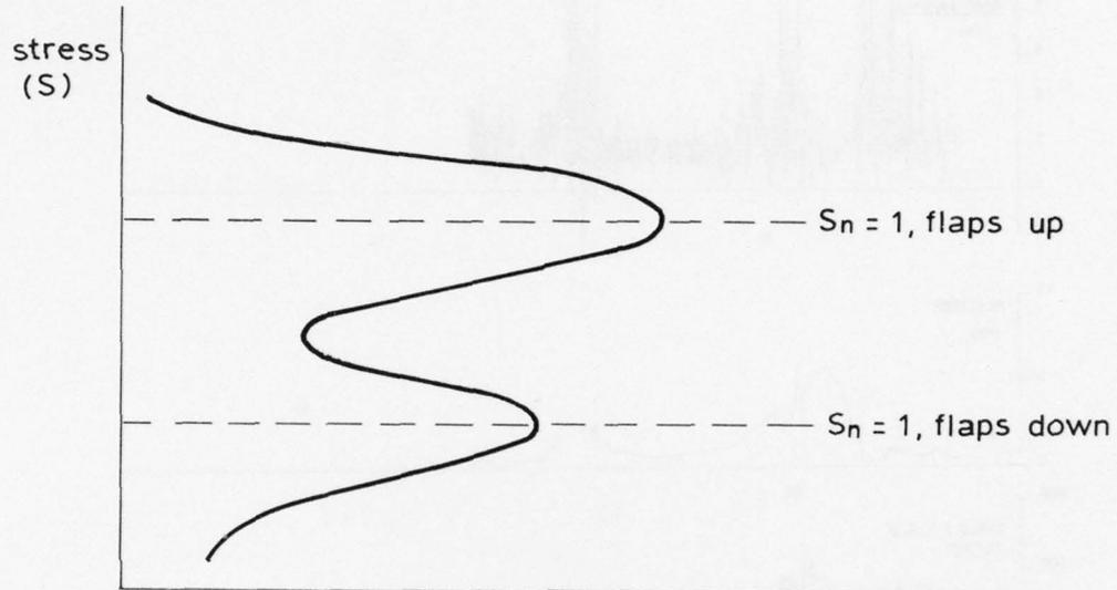
Fig.7.12 Level-cross count result of stabilizer bending stress
