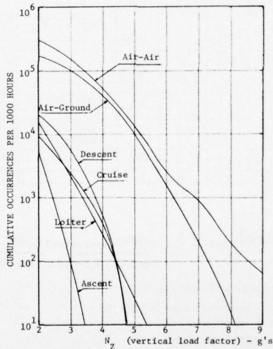
Fig.3.4.3.1 Mission segment positive maneuver spectra (from Reference 1)
