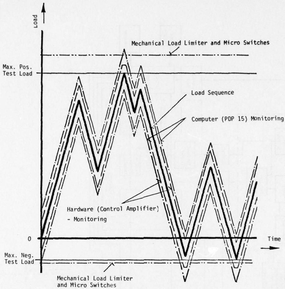
Fig.5.5.3 Continuous jack load monitoring during fatigue testing
