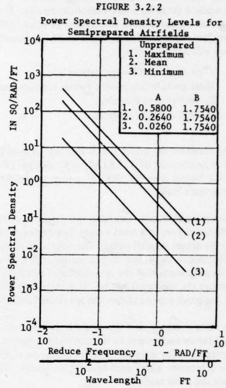
Fig.3.3.2.2 Power spectral density levels for semiprepared airfields
