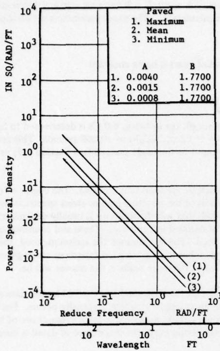
Fig.3.3.2.1 Power spectral density levels for paved airfields
