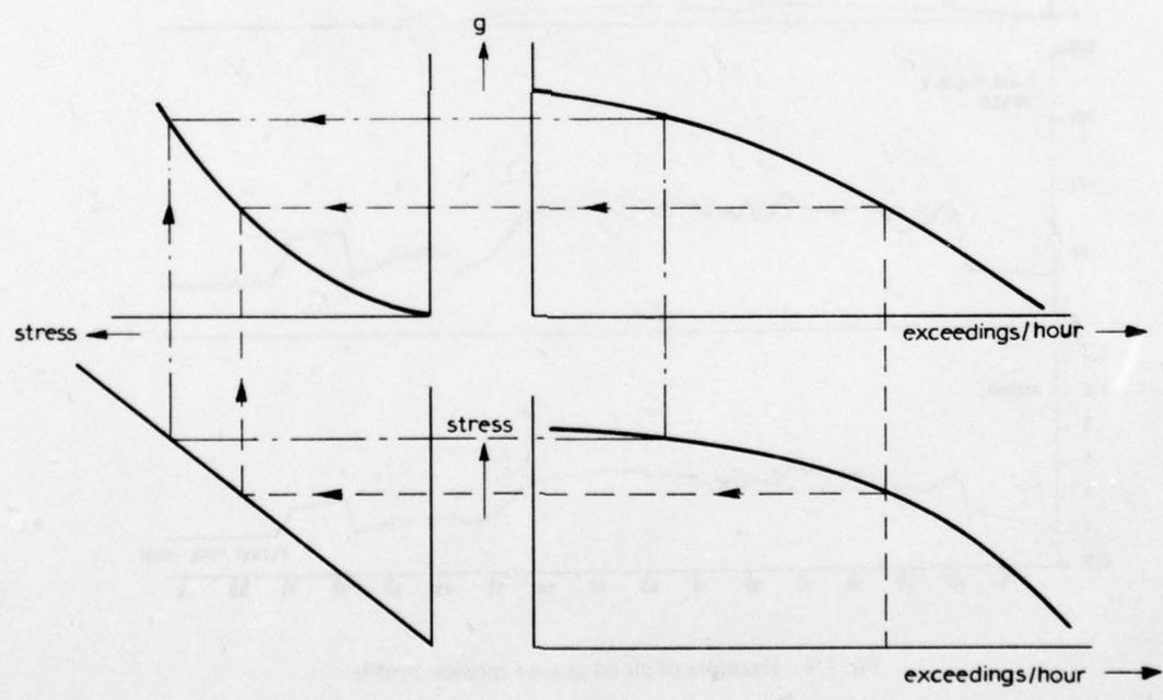
Fig.7.8 Illustration of the spectrum-correlation technique
