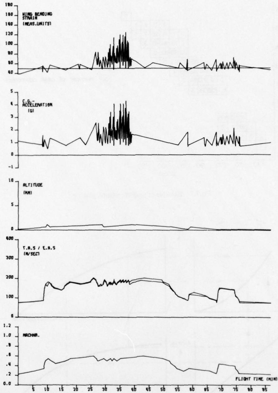
Fig.7.9 Example of air to ground mission profile
