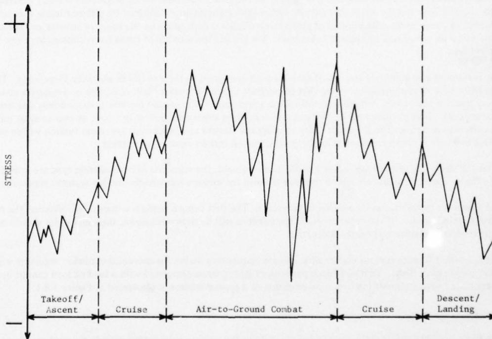
Fig.3.8.1.1 Representation of a mission segment-by-mission segment mission
