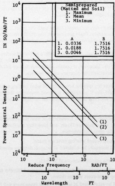
Fig.3.3.2.3 Power spectral density levels for unprepared airfields
