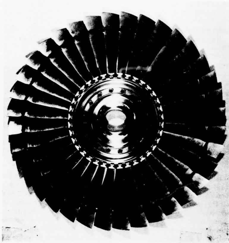
(a) Assembled third stage fan section
