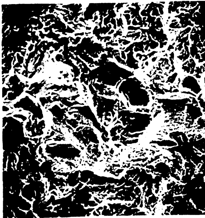
Figure 7. SEM fractograph showing cleavage and intergranular failure modes - 750°F temper - 900X.
