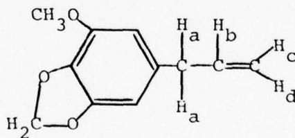
The nmr (cf. Figure IX) is typical of the compound myristicin with a singlet at  $\tau$ 3.62 (aromatic protons), a singlet at  $\tau$ 4.15 (methylenedioxy protons), a multiplet under the singlet at  $\tau$ 4.15 ( $H_b$  coupled with  $H_a$ ,  $H_c$  and  $H_d$ ), a multiplet and poorly defined triplet at  $\tau$ 4.90 and
