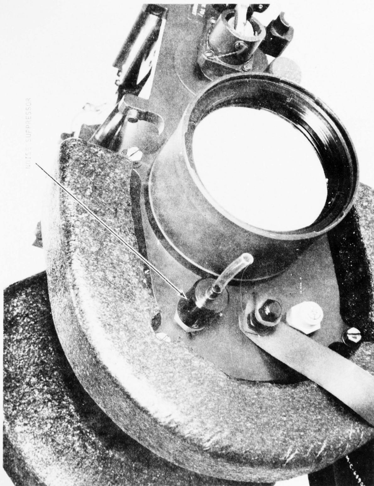
Figure 2-20. APE Model - Coolant Gas Noise Suppressor
