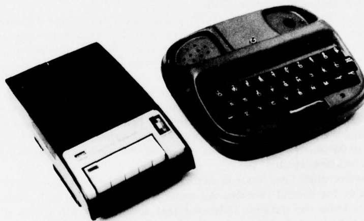
FIGURE 3.—Manual Communication Module showing portable electronic typewriter with built-in acoustic coupler, and scroll cassette unit.
