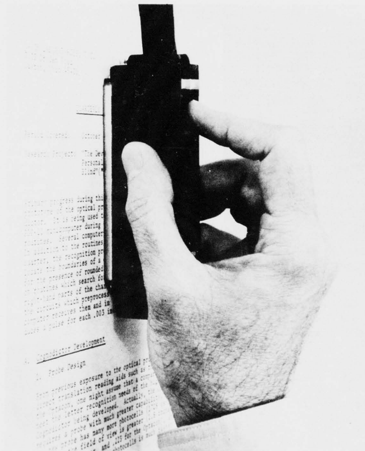
FIGURE 1.—The large field of view (1.5 in high) and long high-friction rollers of the Cognodictor probe make freehand scanning of print easier than ever.
