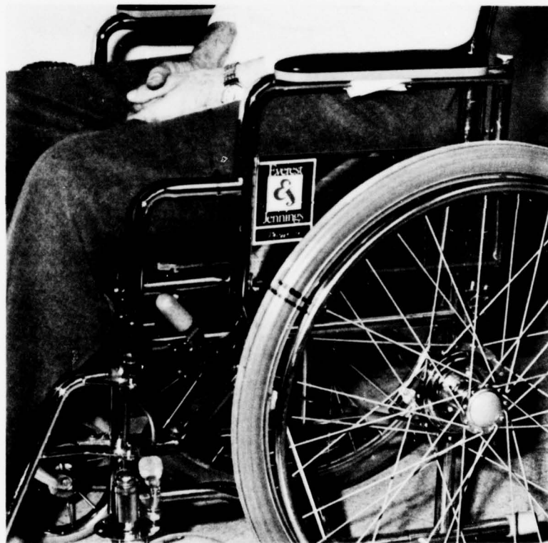
FIGURE 17.—Everest and Jennings Hub-Brake Wheel-Lock System installed on a wheelchair. The brake rod may be connected to the lever to produce a push-to-lock or a pull-to-lock action, as desired.
