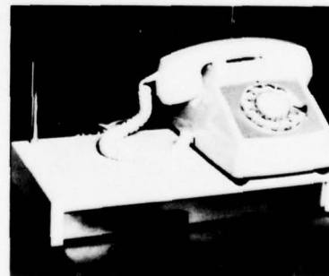
FIGURE 4. (above)—Kari-Fone (rear view) with battery charger. Terminal block at right is intended to permit handling up to five different telephone numbers on a single base unit.
