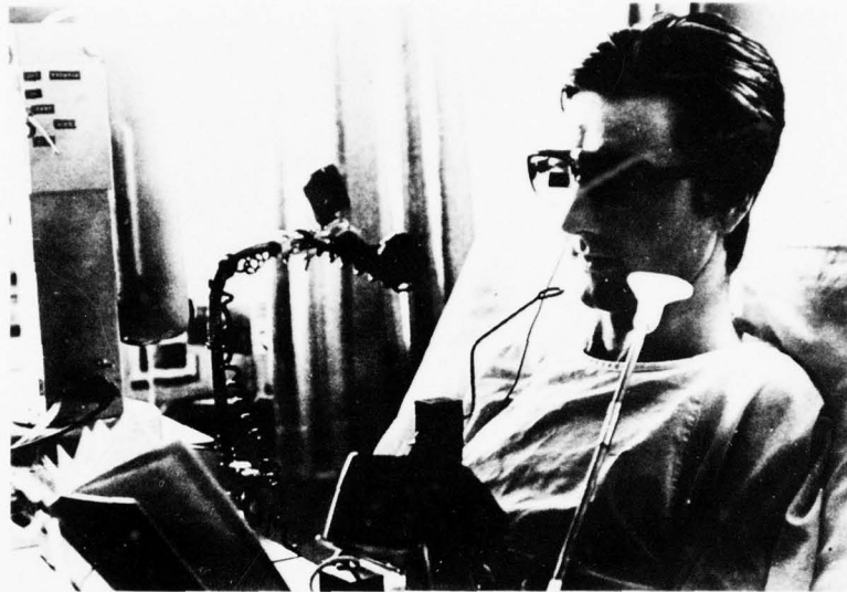
FIGURE 11.—Eyeglasses used to mode-select manipulator motions. A sensing accelerometer is located on the eyeglass frame.
