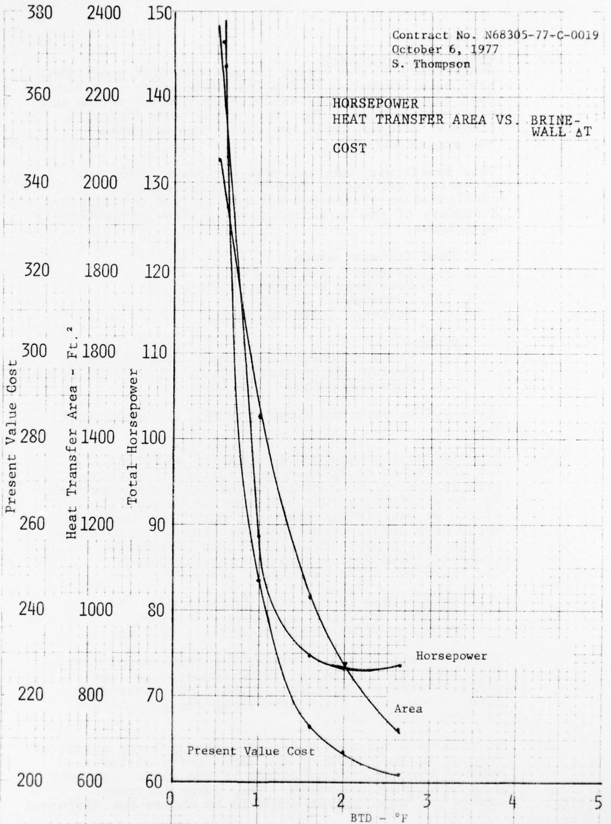
(Temperature Difference Between Brine & Tube Wall)
