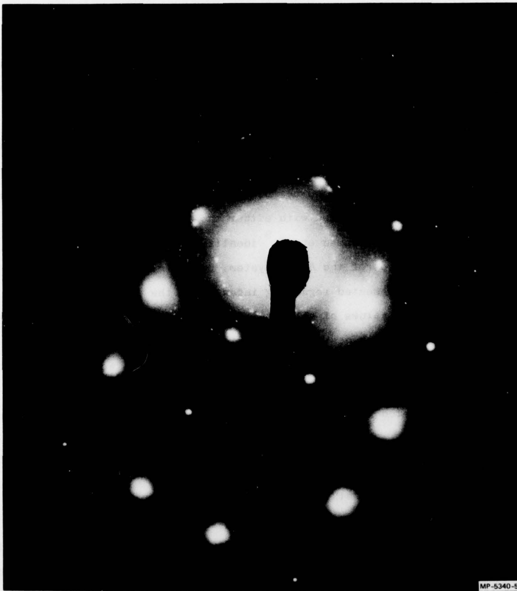
FIGURE 5 TRANSMISSION ELECTRON DIFFRACTION PATTERN OBTAINED FROM MIXING ZONE OF ANNEALED Au/Si STRUCTURE. SUBSTRATE DEPOSITION TEMPERATURE = 50°C; ANNEALED IN AIR FOR 12-HOURS AT 400°C
