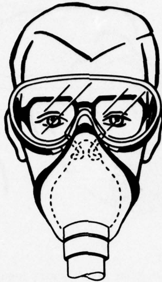
FIGURE 10. Goggles with venting tubes sealed against mask lip.
