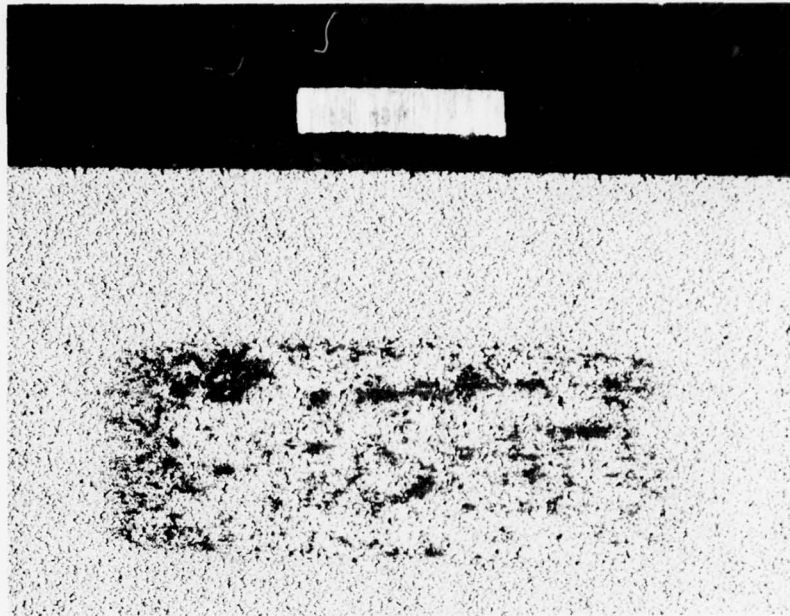
Figure 53: 1800 psi (12.4 MPa) Material A-1 NiCrAl After a 0.030 in (762 \mu m) Rub with an Inconel 600 Blade
