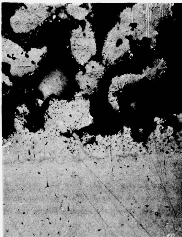
Figure 125: Microstructure of Segment 4 After 100 Thermal Cycles 200X
