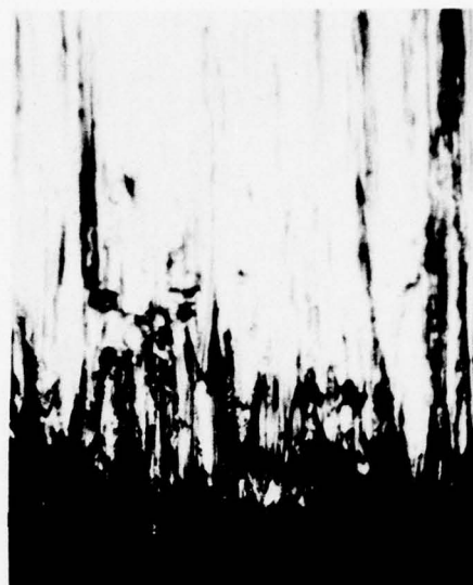
Figure 58: Micrograph of the Leading Edge of an AM 355 Blade Tip After Interaction with Material A-2 NiCrAl. Blade was rotating at 377 ft/sec (115 m/sec) and had an incursion rate of 0.001 in/sec (25 \mu m/sec). 127X
