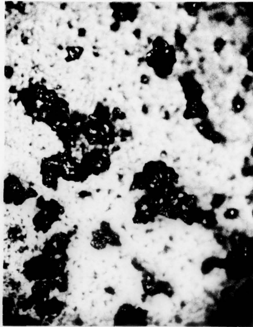
Figure 62: Large Particle Size Debris Collected After Rub Interaction Between AM 355 Blade Tips and Material A-2 NiCrAl 65X
