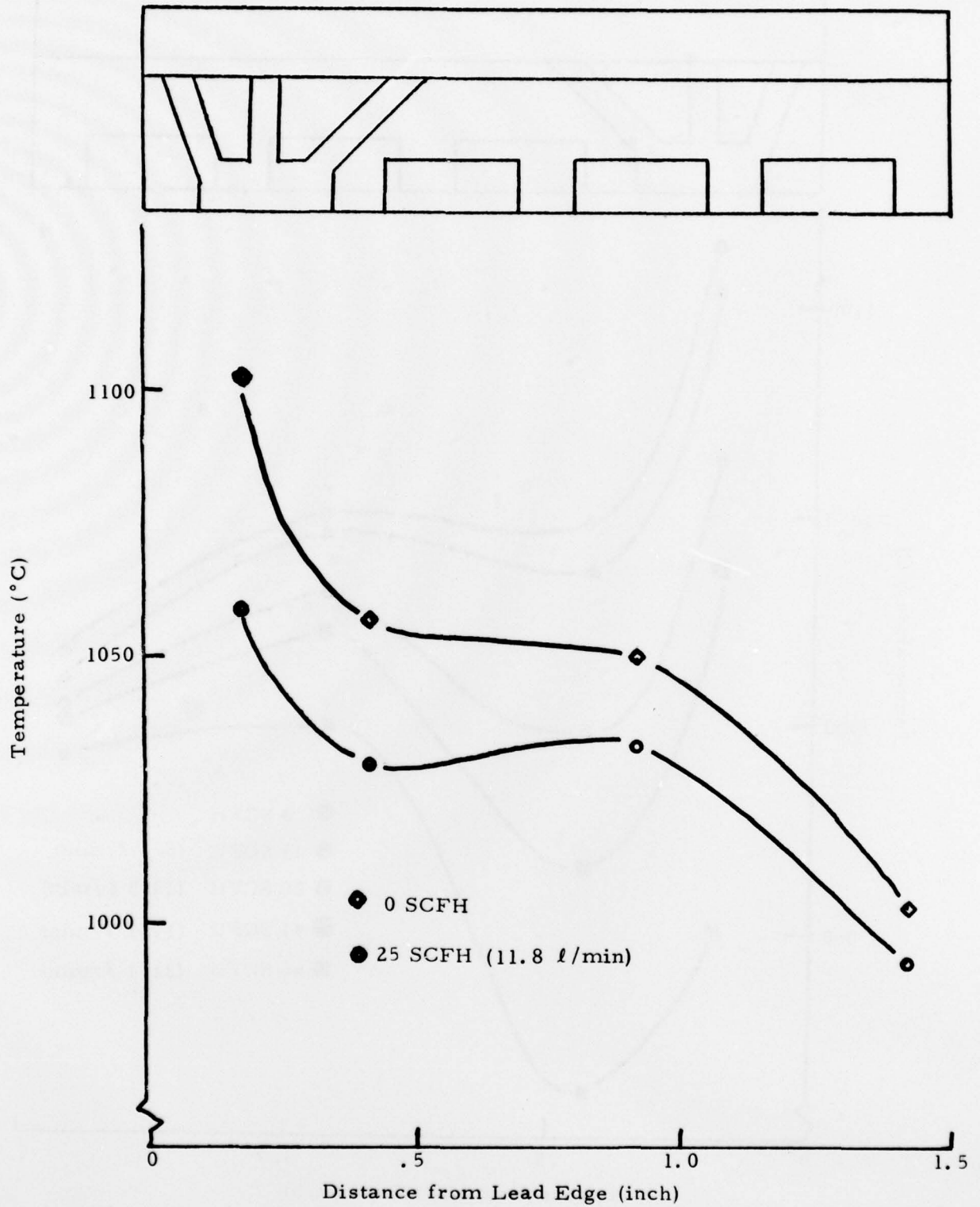
Figure 127: Surface Temperature of Segment 2 as a Function of Position for Different Flow Rates of 1200°F (649°C) Cooling Air
