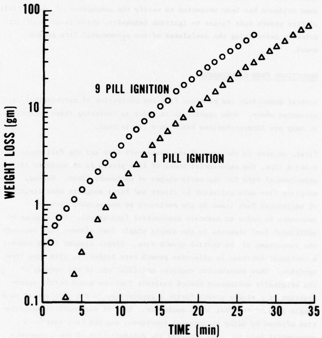
FIGURE 6. COMPARISON OF IGNITION SOURCES, POLYMETHYLMETHACRYLATE SLAB FIRES.
