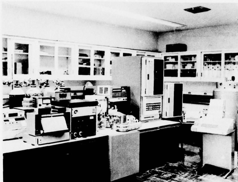
Figure 3. View of the analytical system: Gas chromatograph (Varian 1400)-mass spectrometer (DuPont 21-491)-data acquisition (DuPont 21-094).
