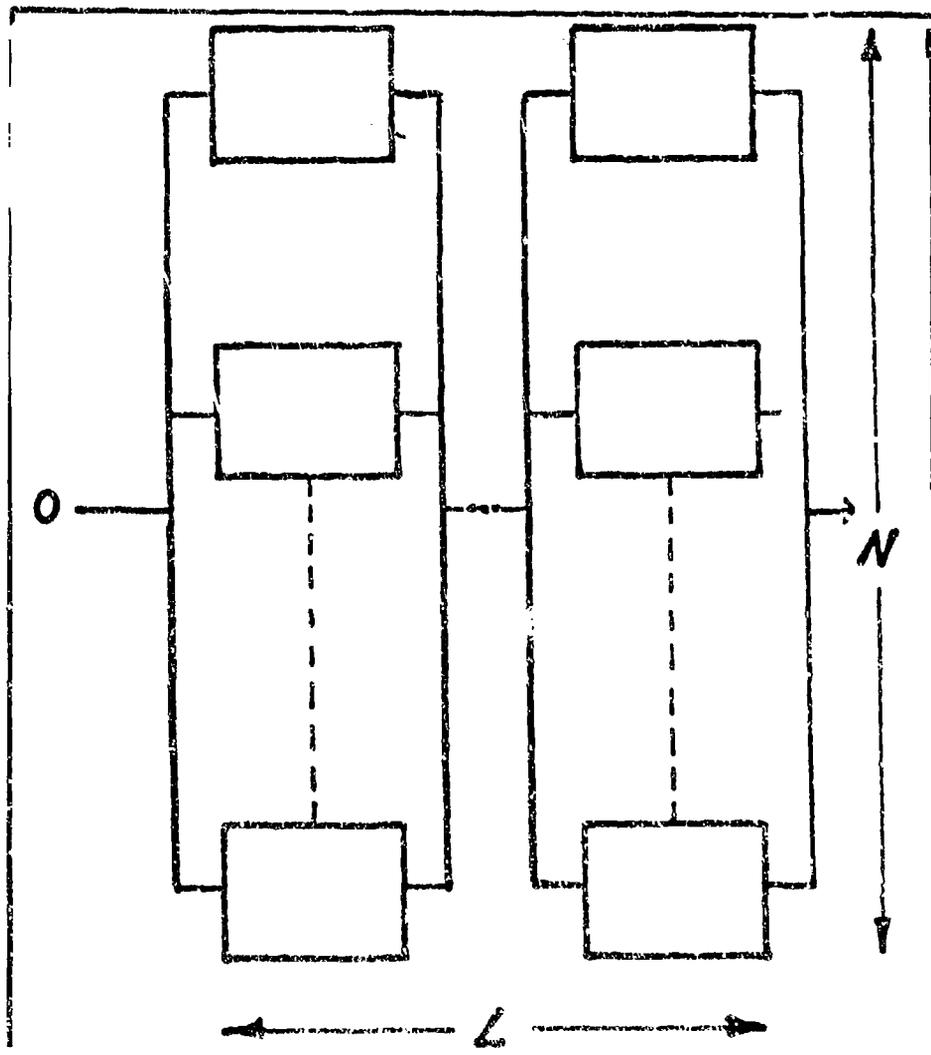
Figure 2.1.  $L$  Redundant Subsystems in Series
