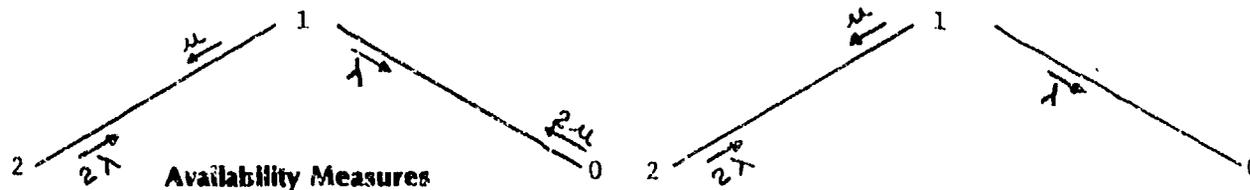
**State Space Diagram For Reliability And Mean Time To Failure Measures**
