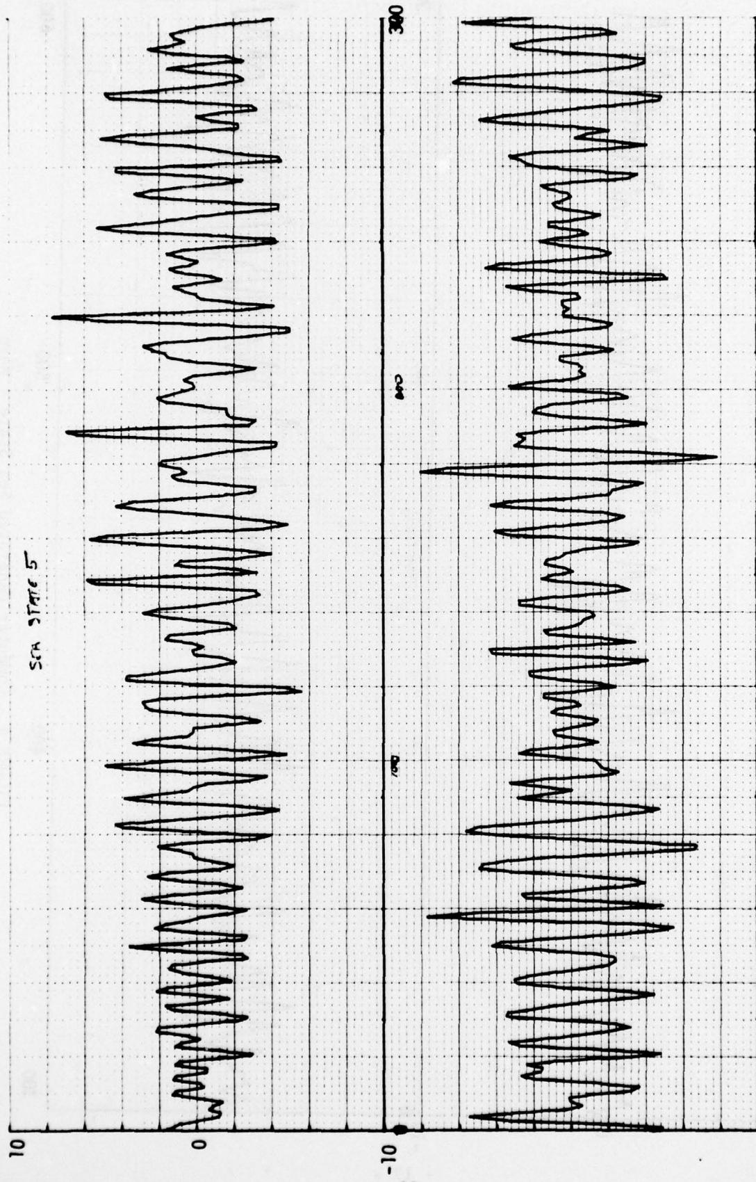
FIGURE 5 - Computer Generated Sea State 5 Wave
