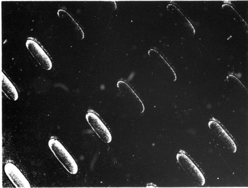
Figure 3: Information pits on surface of videodisc system.
