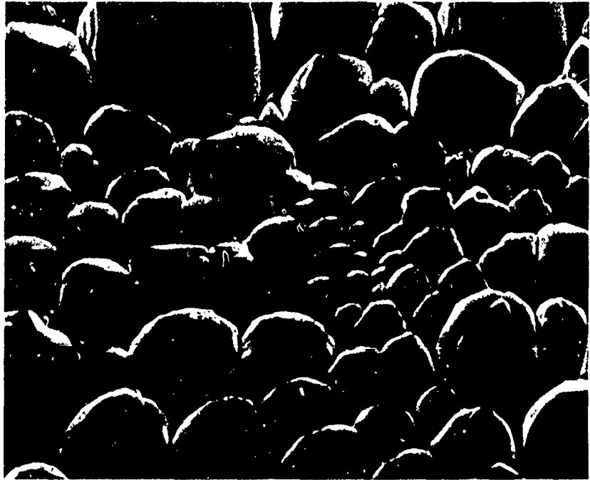
FIGURE 3. SEM Micrograph of Sputtered Bismuth, Same Film as Figure 2, but at 2100X.
