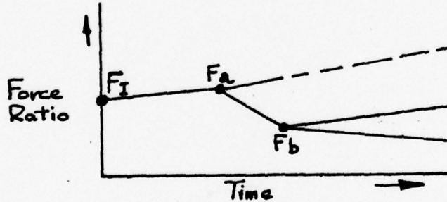
The shape of the curve beyond time (b) depends on the amount of augmentation provided. If a small augmenting force is applied the force ratio will continue to increase. If a large augmenting force is applied the force ratio will decrease.
