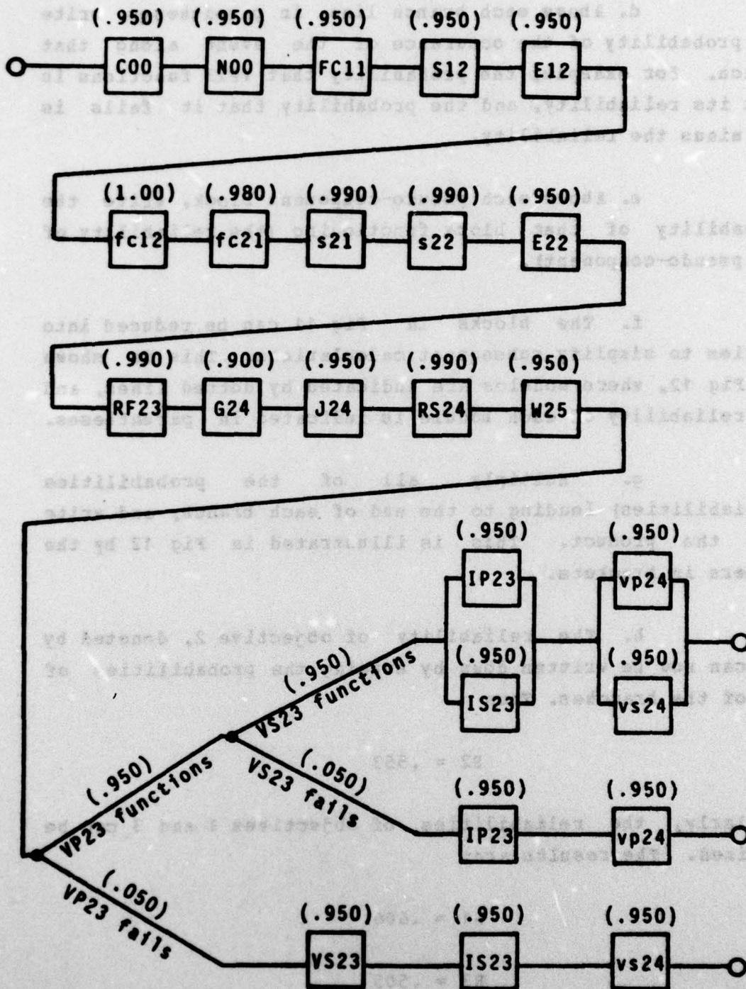
Figure 11 - PIVOTAL DECOMPOSITION OF OBJECTIVE 2
