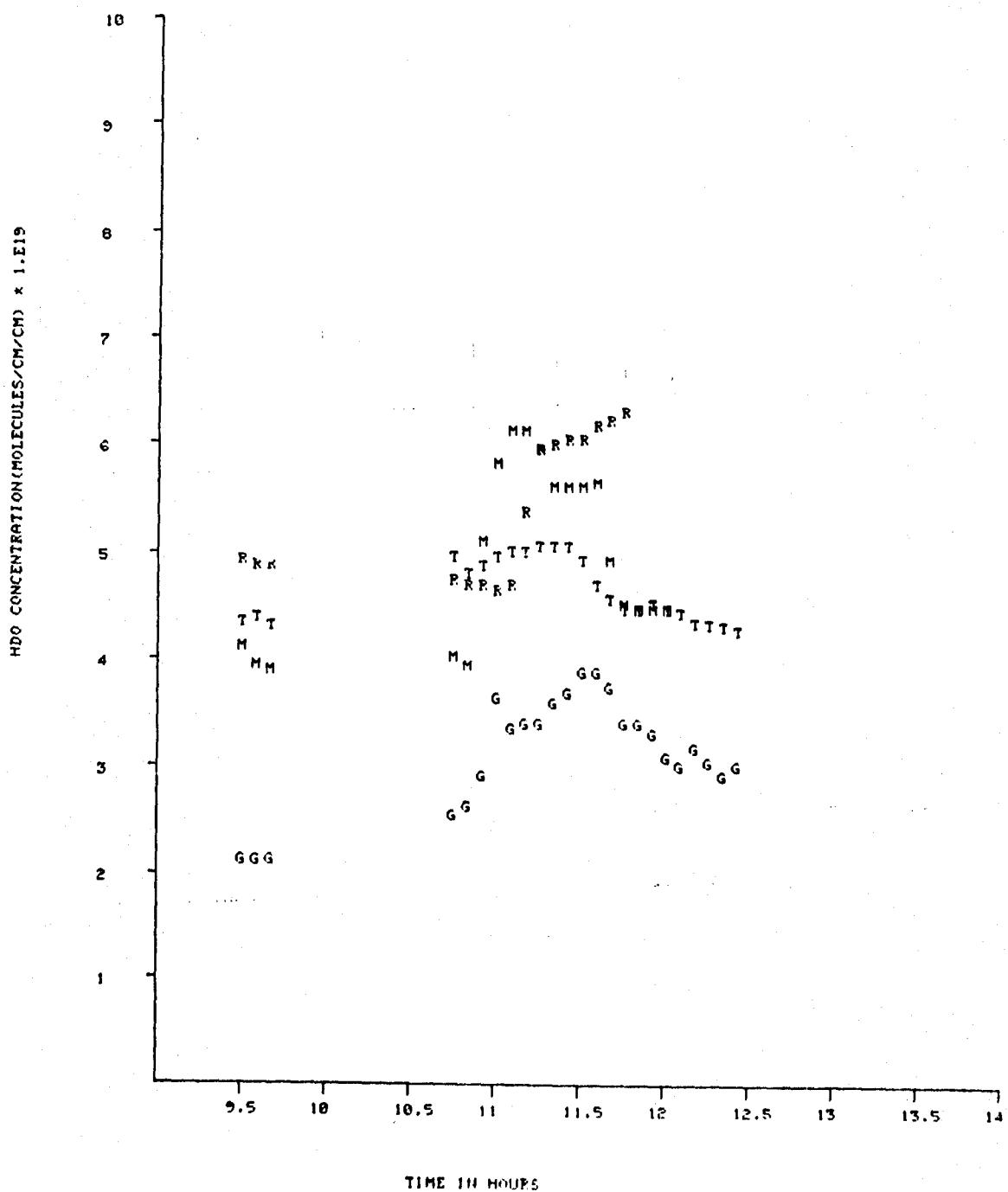
Fig. 5.11 INTEGRATED HDO CONCENTRATION(MOLECULES/CM/CM) FOR 5.12 KM PATH, 31-MAR-77, CCAFS
