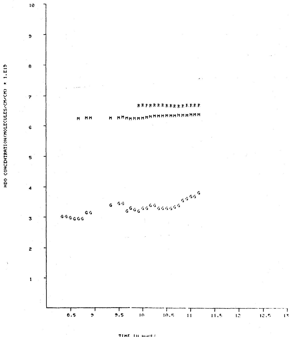
**Fig. 5.7 INTEGRATED HDO CONCENTRATION(MOLECULES/CM/CM) FOR 5.12 KM PATH, 11-MAR-77. COAFS
