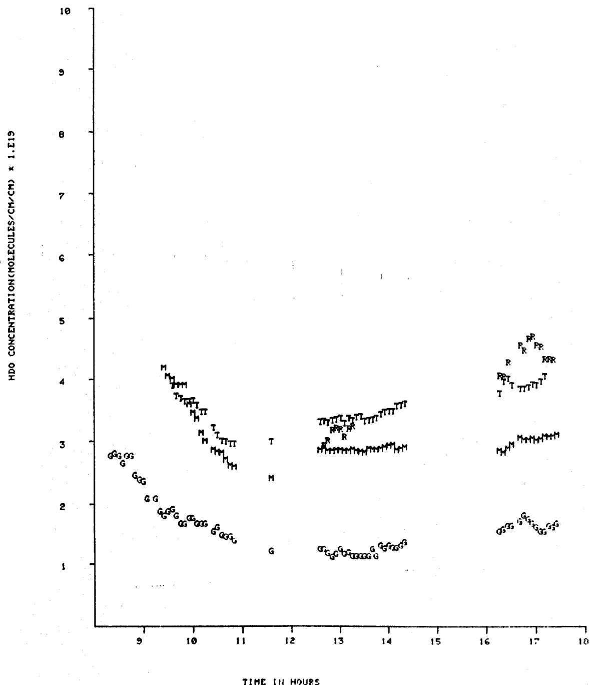
**Fig. 5.10 INTEGRATED HDO CONCENTRATION(MOLECULES/CM/CM) FOR 5.12 KM PATH, 15-MAR-77, CCAFS
