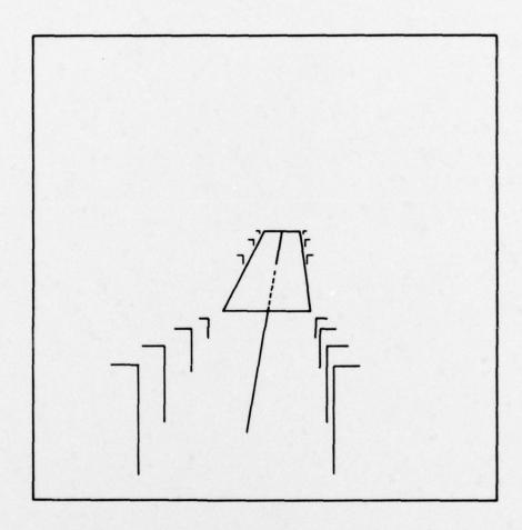
Figure 2. VLD with runway, extended centerline and approach and flare guidance cues.
