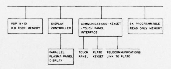
Figure 1. Block diagram of intelligent PLATO terminal for air combat tactics decision training.
