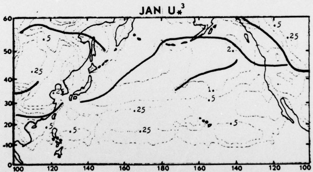
Figure 3. Monthly mean friction velocity cubed ( $u_*^3$ ) from unfiltered  $u$  and  $v$  wind components. Solid heavy lines denote mid-latitude maximums. Contour values are .25, .5, 1., 2., 3., ....  $\times 10^5$  (cm/sec)<sup>3</sup>.
