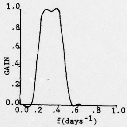
Figure 1. The amplitude of the 31 point band pass filter as a function of frequency. From Blackmon (1976).
