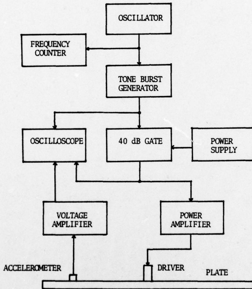
Figure 3. Pulse Measurement Apparatus
