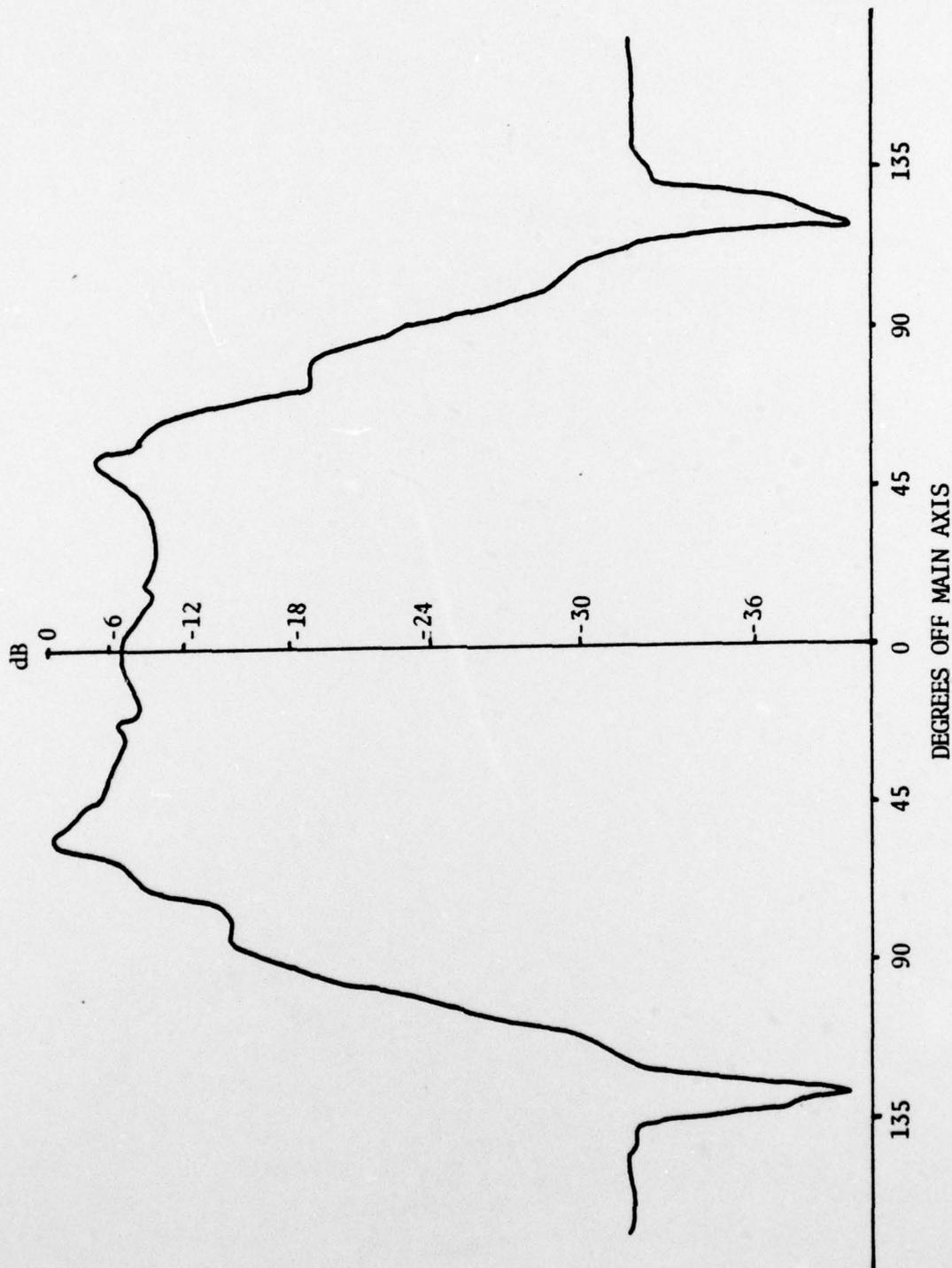
Figure 30. Radiation Pattern - 55 kHz/4 Cycle Pulse
