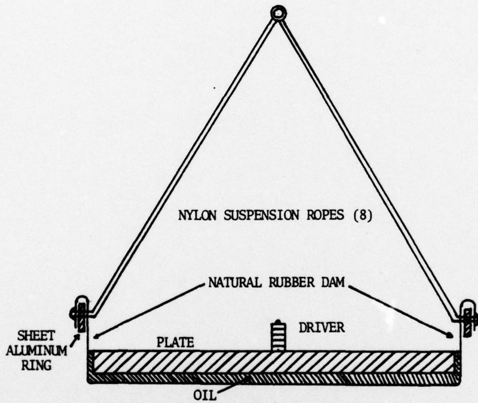
Figure 7. Plate Suspension Apparatus (not to scale)
