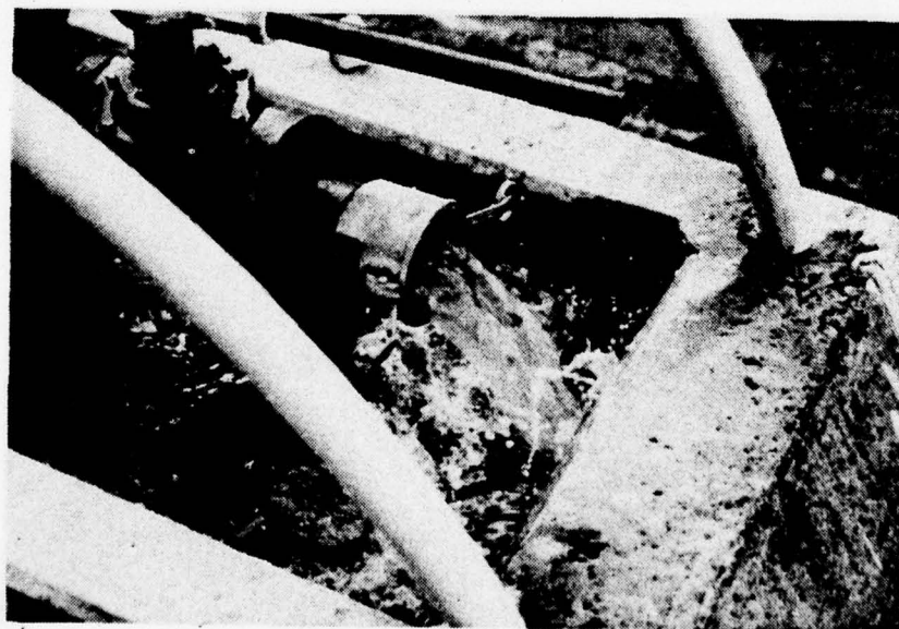
FIGURE 32 BACKFLOW FROM LAST MANIFOLD PIER RISER (TABLE 8 - OPEN RISER NO. 4)
