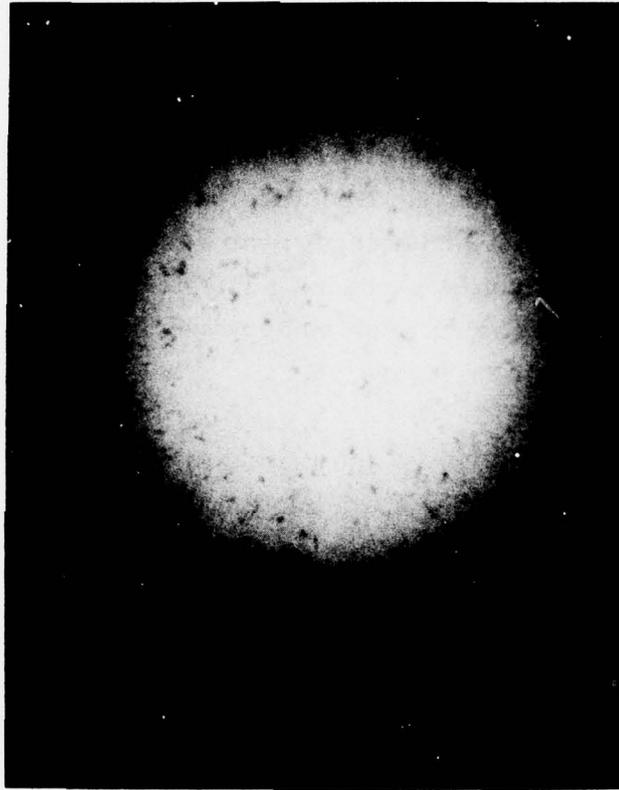
Figure 30. Infrared Microscopy of CVD CdTe Showing Residual Voids (100 $\times$  magnification)
