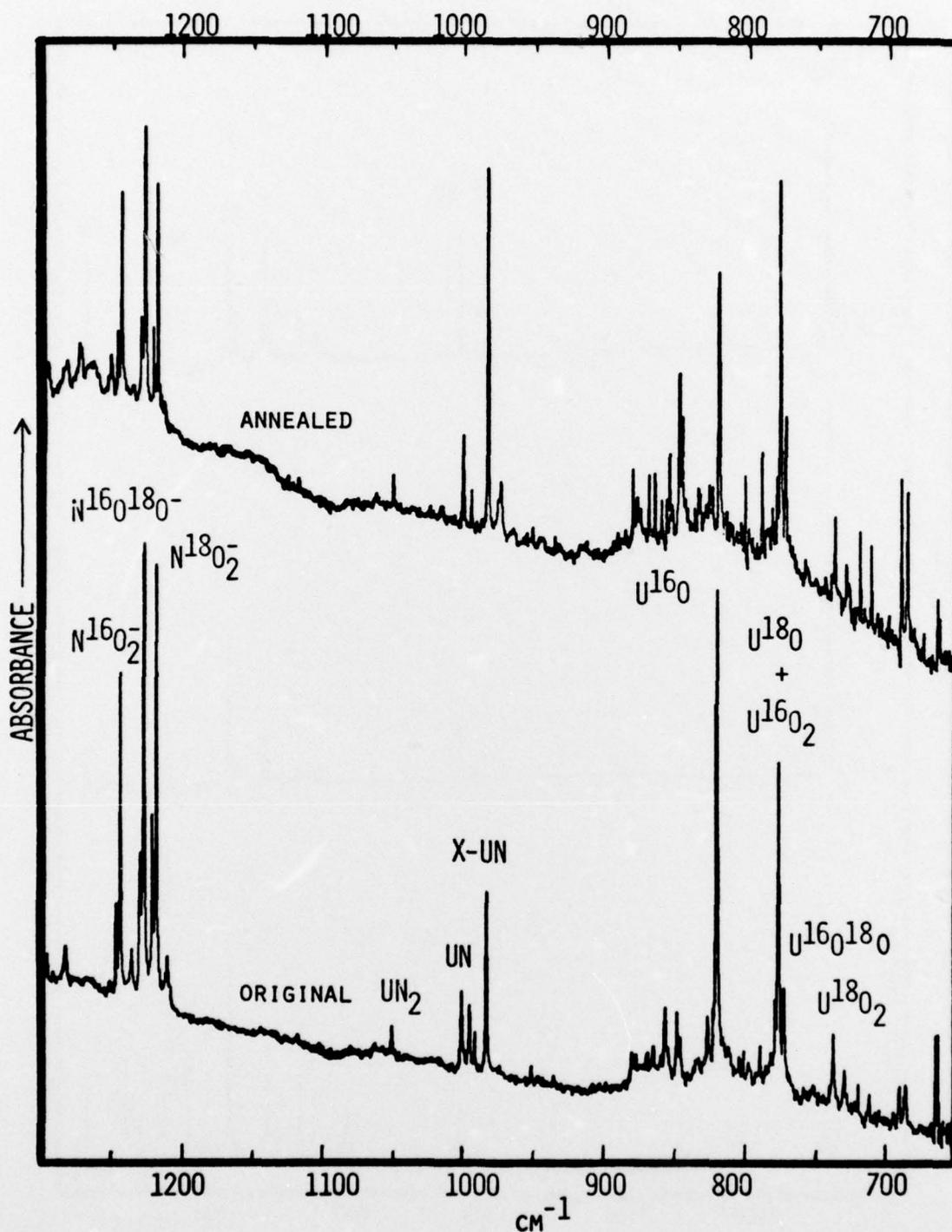
Fig. 6. Infrared spectra of an Ar matrix at 14 K made by cocondensing U atoms with 50%  $^{18}\text{O}$ -enriched  $\text{NO}_2$  (0.1% in Ar). Bottom - the original matrix; and top - after annealing the matrix to 30 K and recooling to 14 K.
