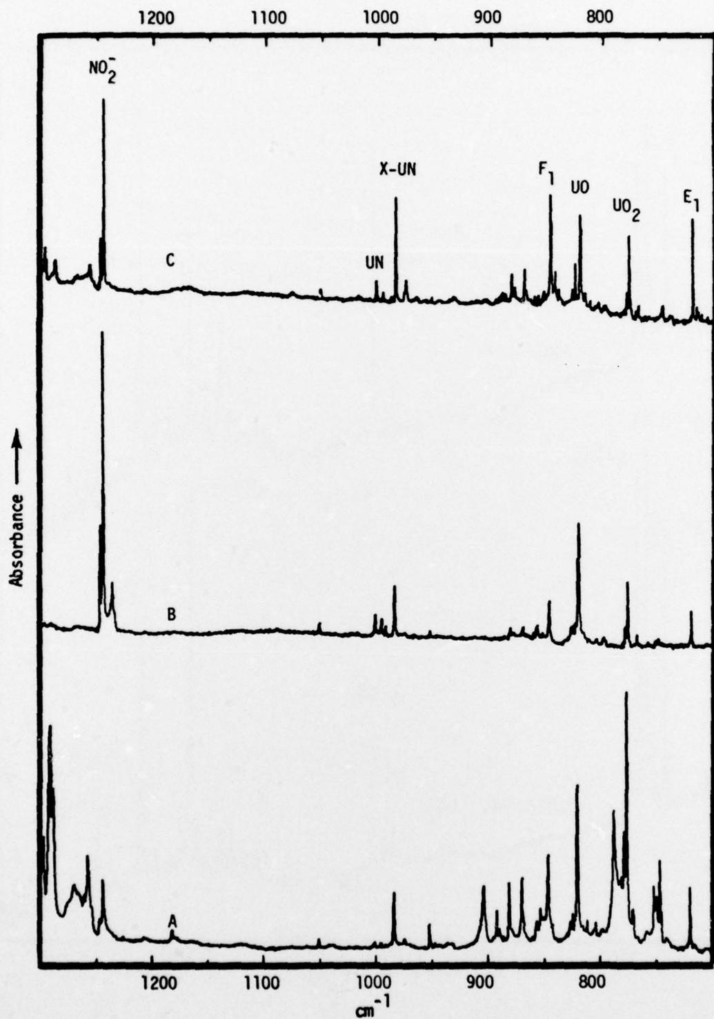
Fig. 5. Infrared spectra of U + NO<sub>2</sub> reaction products in Ar matrices at 14 K. (A) 1% <sup>14</sup>N<sup>16</sup>O<sub>2</sub> in Ar; (B) 0.1% <sup>14</sup>N<sup>16</sup>O<sub>2</sub> in Ar; (C) annealed matrix containing 0.1% <sup>14</sup>N<sup>16</sup>O<sub>2</sub>.
