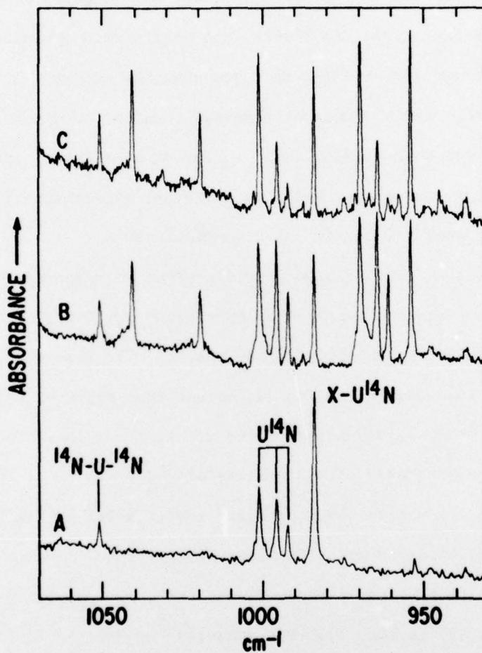
Fig. 3. Infrared spectra obtained from an Ar matrix at 14 K. (A) The products of cocondensation of U atoms with  $\text{NO}_2$ ; (B) the products of sputtering U with a 1:1:800  $^{14}\text{N}_2$ :  $^{15}\text{N}_2$ : Ar mixture; (C) the same matrix as (B) after annealing to 30 K and recooling to 14 K.
