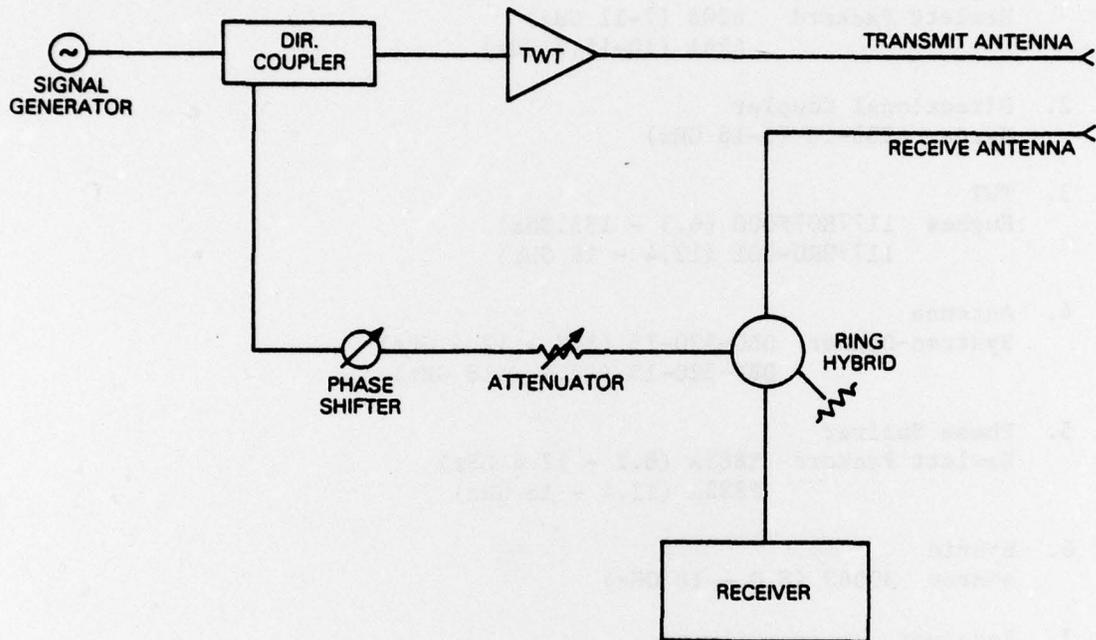
Fig. 1 — Schematic diagram cw chaff measurement system
