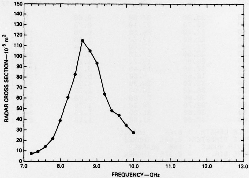
Fig. 4 - RCS (0.66 in. chaff dipole) vs frequency
