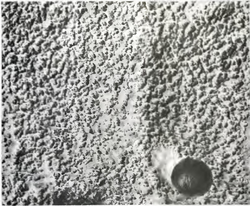
Fig 13 Sealed chromic-acid anodized surface (33,000 x magnification)
