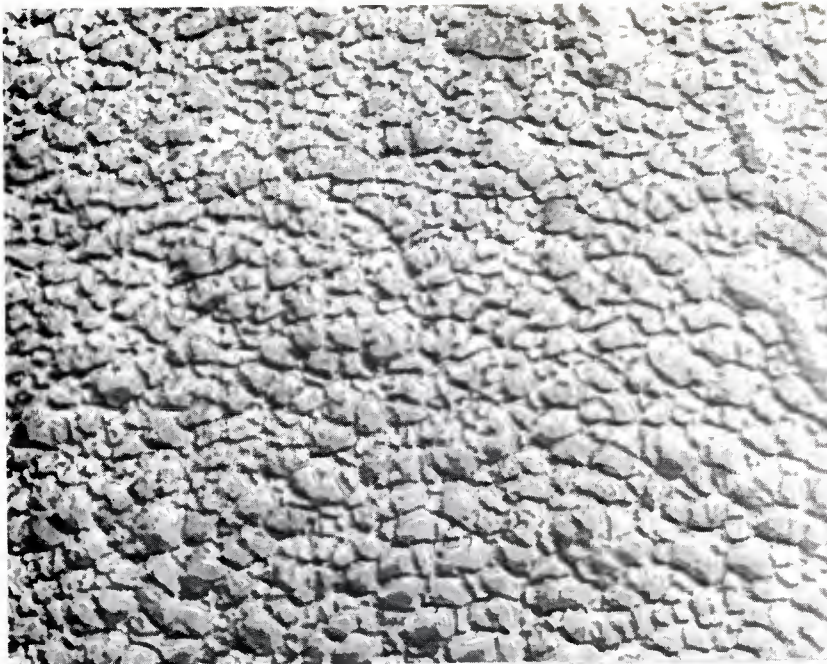
Fig 6 TEM of (FPL) deoxidized surface (100,000 x magnification)
