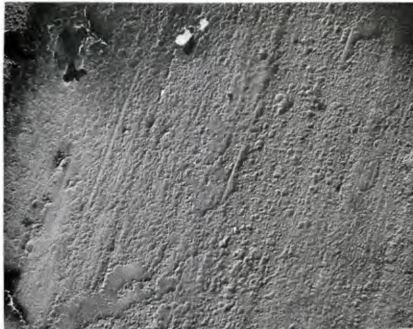
Fig 1 TEM of acetone-degreased surface (6,750 x magnification)
