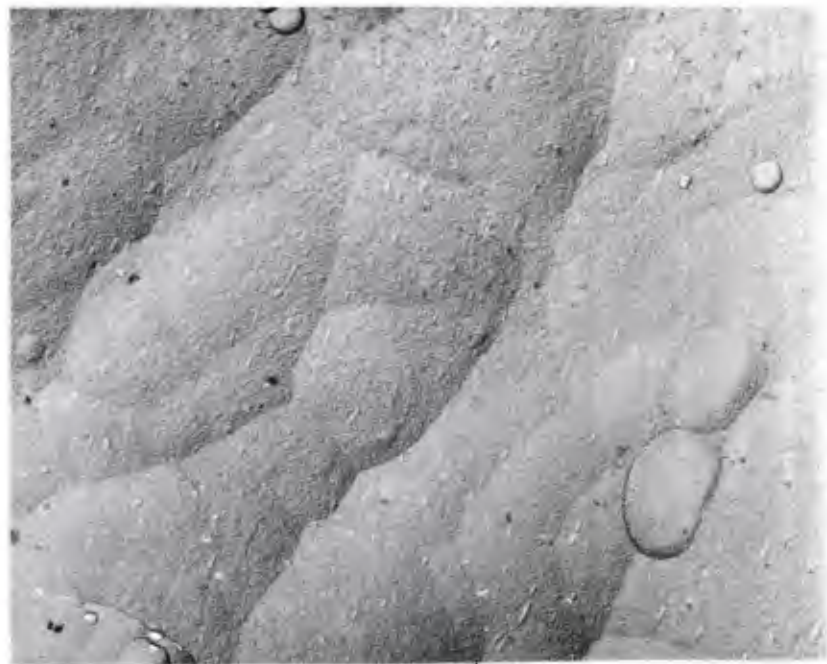
Fig 5 TEM of (FPL) deoxidized surface (6,750 x magnification)
