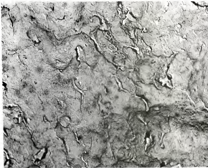
Fig 3 TEM of alkaline -cleaned surface (6,750 x magnification)
