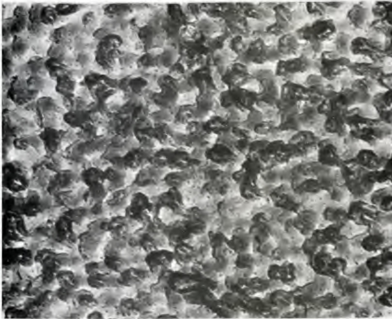
Fig 12 Sealed chromic-acid anodized surface (70,000 x magnification)
