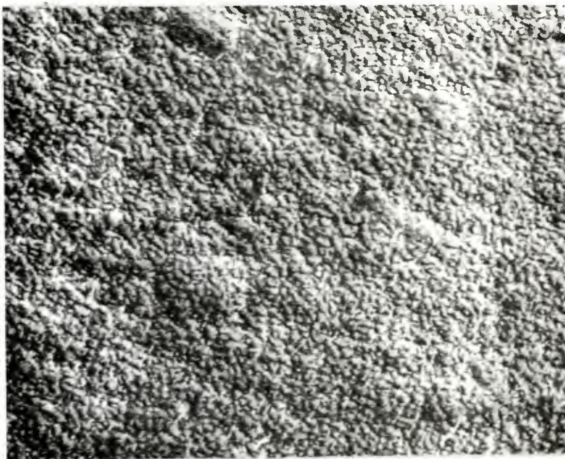
Fig 8 Surface chromic-acid anodized for 2½ minutes at 7½ volts (100,000 x magnification)
