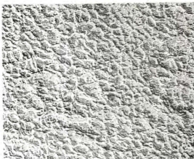
Fig 7 TEM of surface chromic-acid anodized for 2 minutes at 7½ volts (100,000 x magnification)
