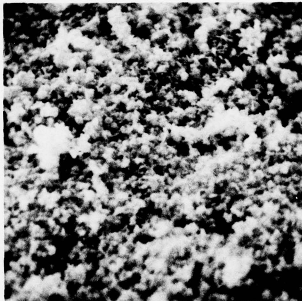
Figure 11. SEM micrograph of a silver metal deposit on human molar enamel. The enamel had been etched for 1.0 minute with 42.5% H_3PO_4 , then rinsed. Plating sequence [AgF 100 gpl, pH 6.5 - FeSO_4 saturated solution + .1 gpl SnF_2 , pH6.] 10 repetitions. Magnification 3000X.
