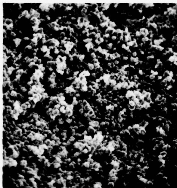
Figure 2. SEM micrograph of a silver metal deposit human molar enamel. The enamel had been etched for 1.0 minute with 42.5% H_3PO_4 , then rinsed. Plating sequence [AgF 100 3 gpl, pH6.5- FeSO_4 saturated solution, pH 3.5] 10 repetitions. Magnification 1000X.
