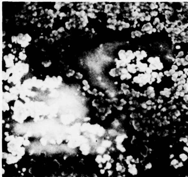
Figure 5. SEM micrograph of human molar enamel partially covered with silver. The enamel had been etched for 1.0 minute with 42.5% H_3PO_4 . Plating sequence [ AgNO_3 , 100gpl, pH4- FeSO_4 , 300gpl, pH 2] 10 repetitions. The very light areas are nonadherent silver particles. Magnification 1000X.
