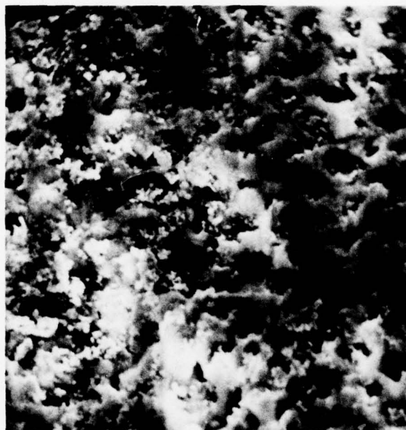
Figure 1. SEM micrograph of human molar enamel partially covered with silver. The enamel had been etched for 1.0 minute with 42.5% H_3PO_4 , and then rinsed. Plating sequence (A F^{4.25} gpl, pH6.5- FeSO_4 , saturated solution, pH 6 3.5) 10 repetitions. 4 Magnification 1000X
