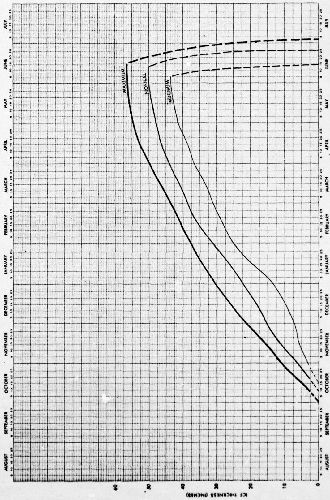
FIGURE 168 MALYYE KARMAK BAY THEORETICAL ICE GROWTH AND ESTIMATED DISINTEGRATION CURVES
