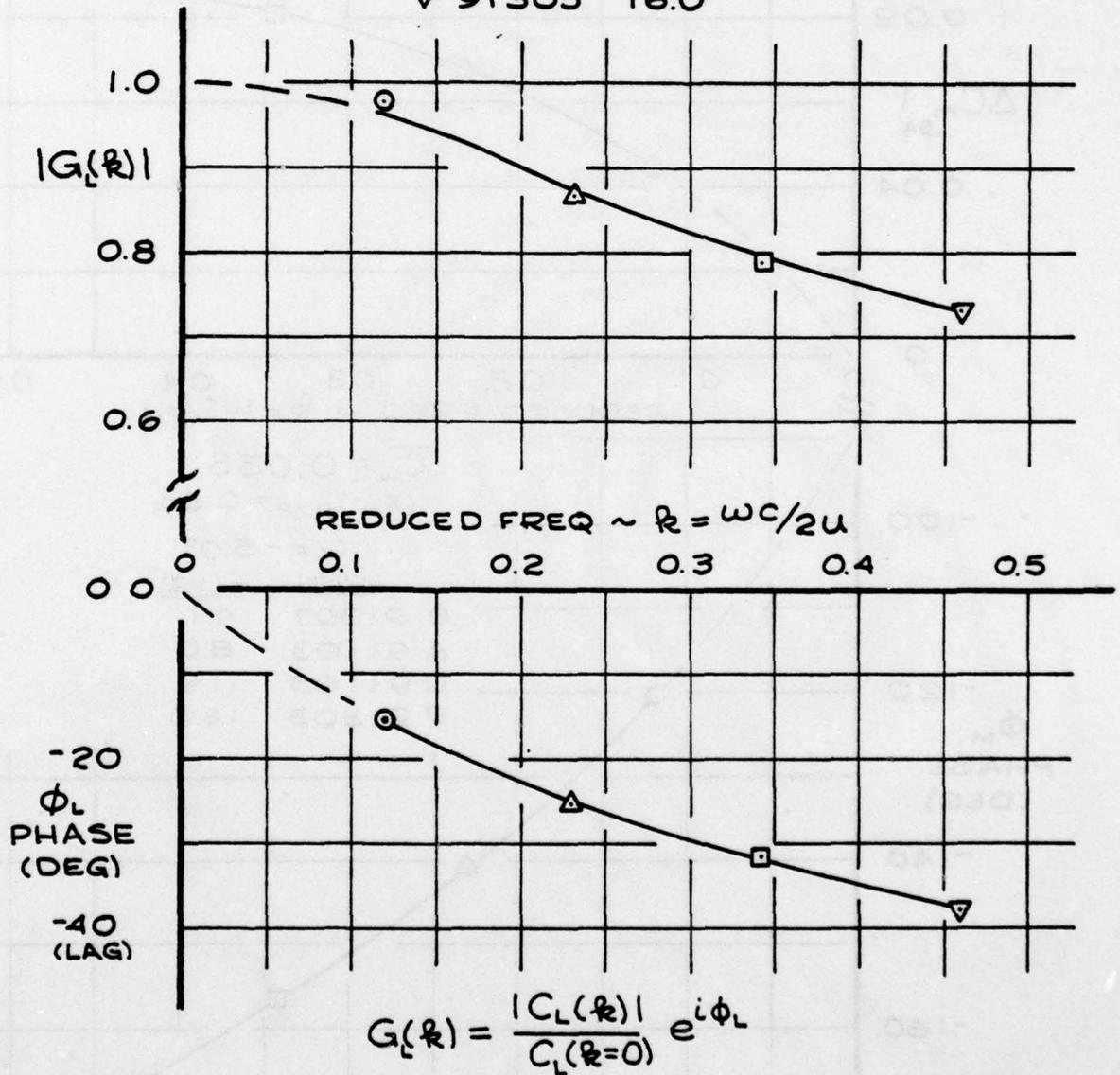
FIG. 6: CIRCULATION CONTROL LIFT TRANSFER FUNCTION
