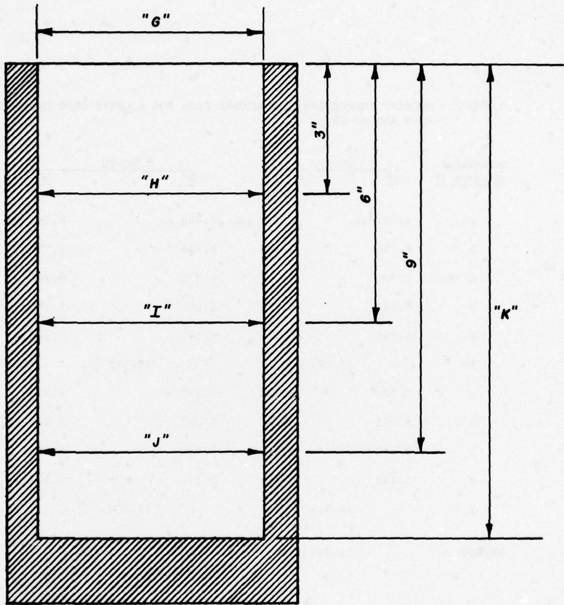
FIGURE 7B. INTERIOR DIMENSIONAL DATA LOCATIONS FOR SQUEEZE CAST CYLINDERS SC-9 AND SC-10.
