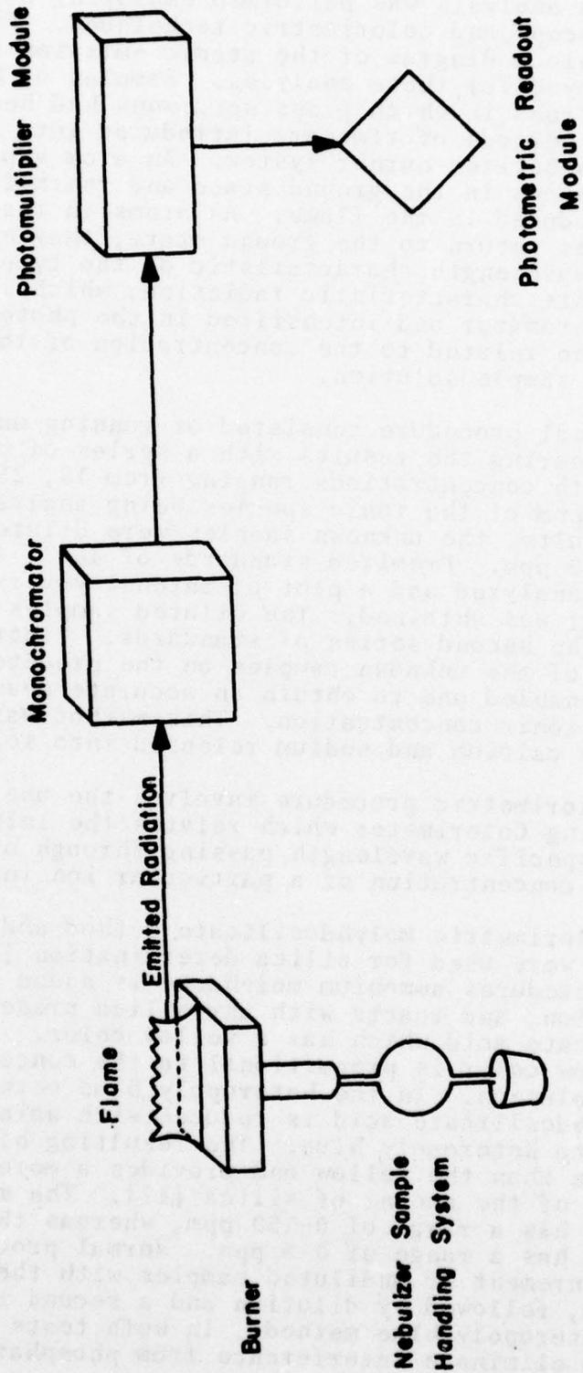
Figure 1. Schematic block diagram of the atomic emission spectrophotometer employed for solution analyses.
