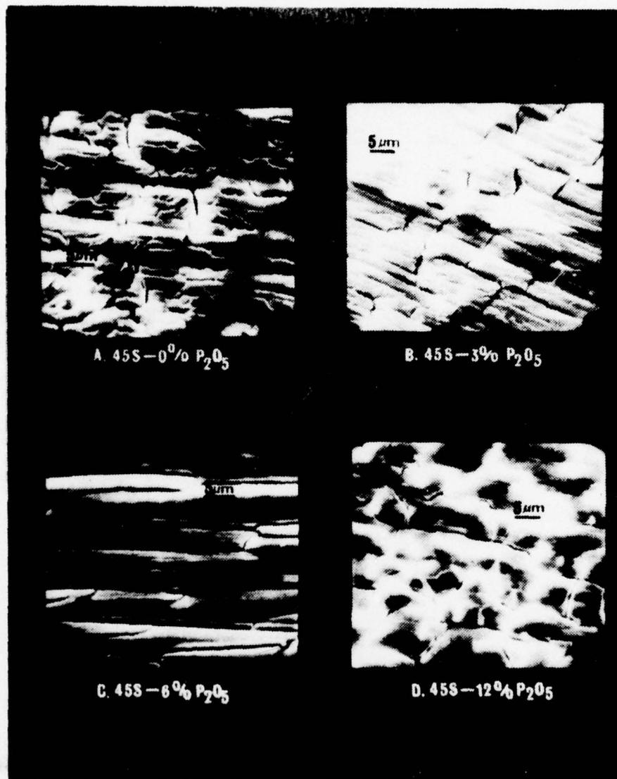
Figure 12. Scanning electron micrographs of corroded surface of bioglass compositions. (A) 45S-0%  $P_2O_5$ , (B) 45S-3%  $P_2O_5$ , (C) 45S-6%  $P_2O_5$ , (D) 45S-12%  $P_2O_5$ . Samples were corroded for one hour in an aqueous solution buffered at pH of 7.4 and maintained at 37°C. The surfaces were ground with dry 600 grit SiC prior to the corrosion treatment.
