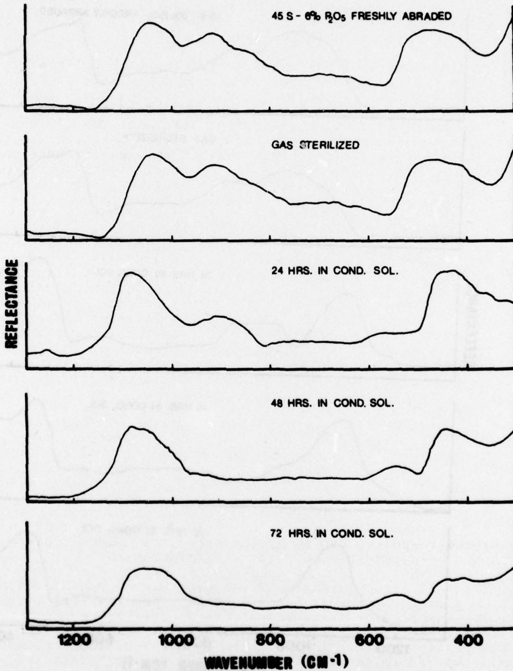
Figure 2. Changes in infrared reflection spectrum of 45S-6% P<sub>2</sub>O<sub>5</sub> glass during conditioning treatment.
