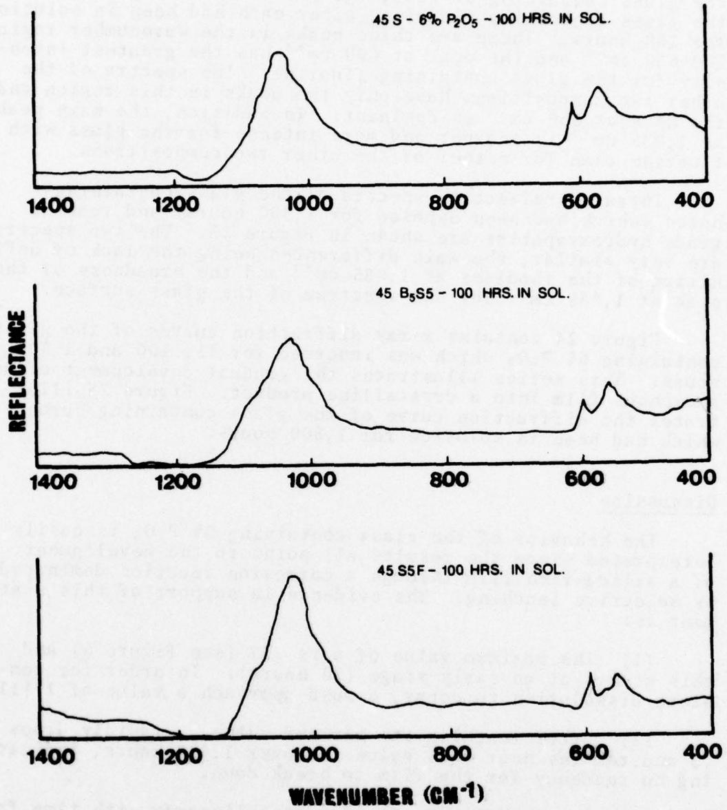
Figure 22. A comparison of the infrared reflection spectra of the bioglasses 45S-6% P<sub>2</sub>O<sub>5</sub>, 45B<sub>5</sub>S<sub>5</sub> and 45S<sub>5</sub>F after a corrosion treatment of 100 hours in an aqueous solution buffered at pH 7.4 and maintained at 37°C.
