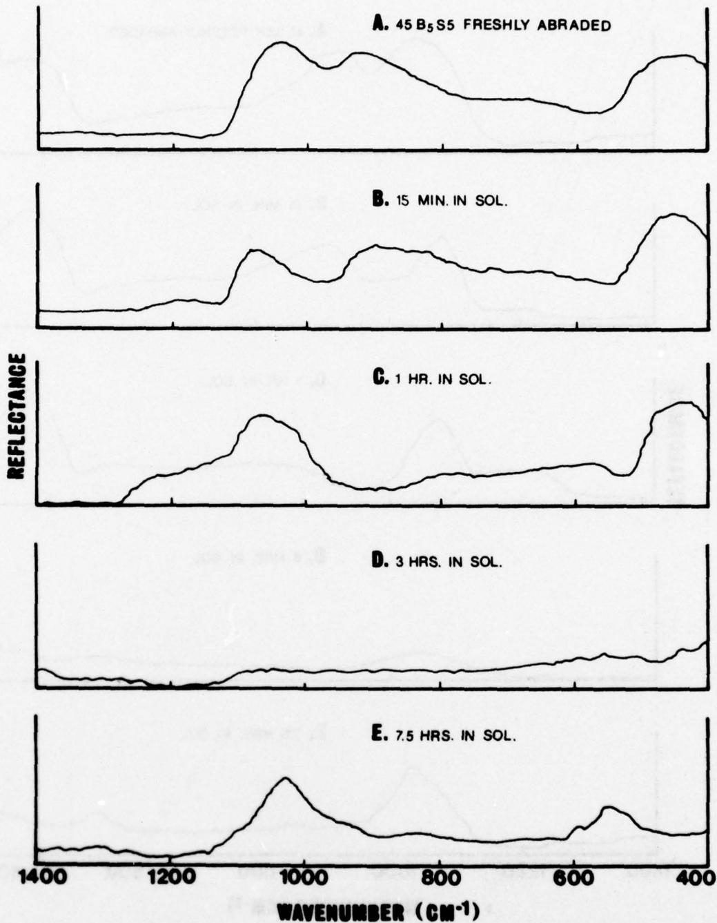
Figure 20. Changes in infrared reflection spectrum of the bioglass 45B<sub>5</sub>S<sub>5</sub> as a function of corrosion time.
