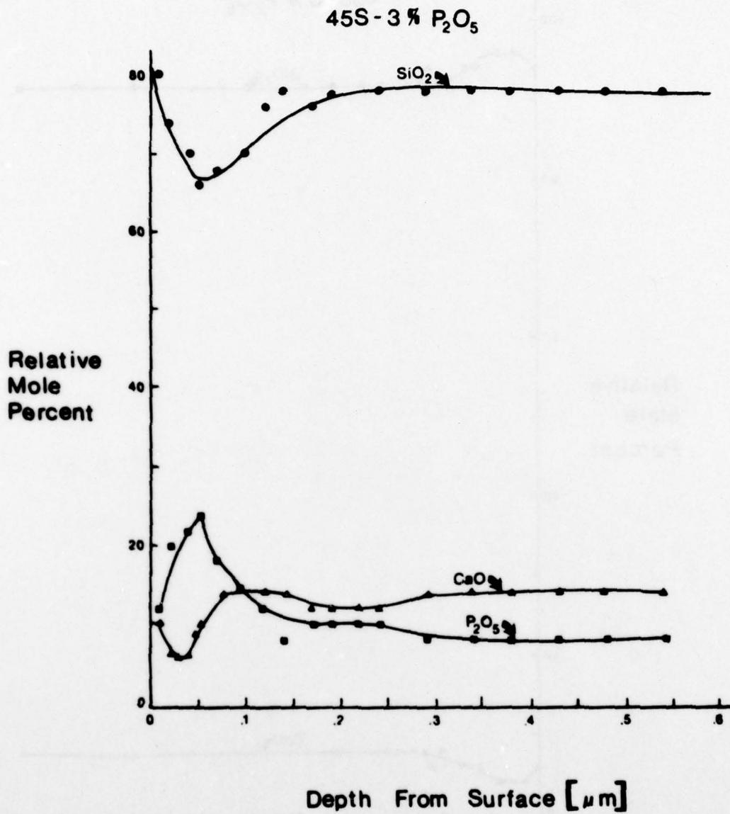
Figure 9. Chemical profile expressed in mole percent of a 45S-3% P<sub>2</sub>O<sub>5</sub> bioglass corroded one hour at 37°C and pH = 7.4.
