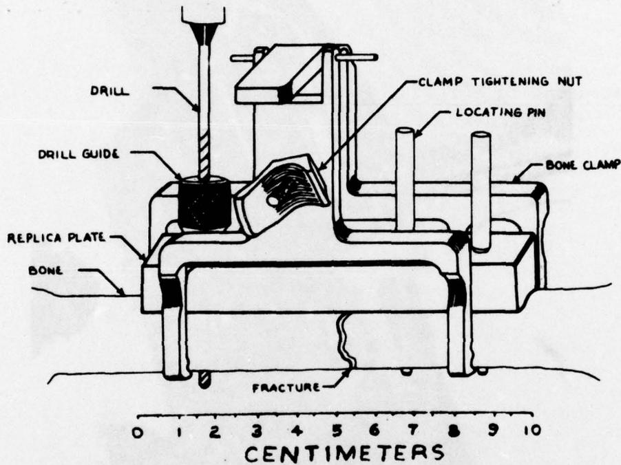
Figure 7. The clamp holds both bone fragments in alignment while the four screw holes are drilled, using the metal replica plate as a template. The locating pins are inserted into the drilled holes to prevent shifting of the plate during the subsequent drilling.
