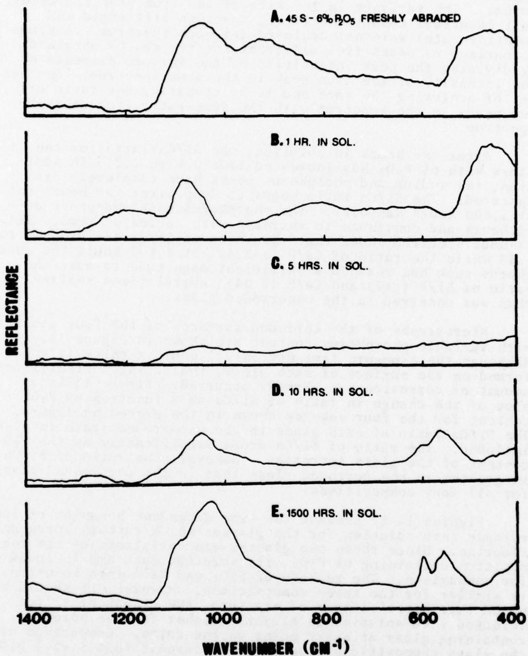
Figure 10. Changes in infrared reflection spectrum of bio-glass composition 45S-6% P<sub>2</sub>O<sub>5</sub> as a function of corrosion time.
