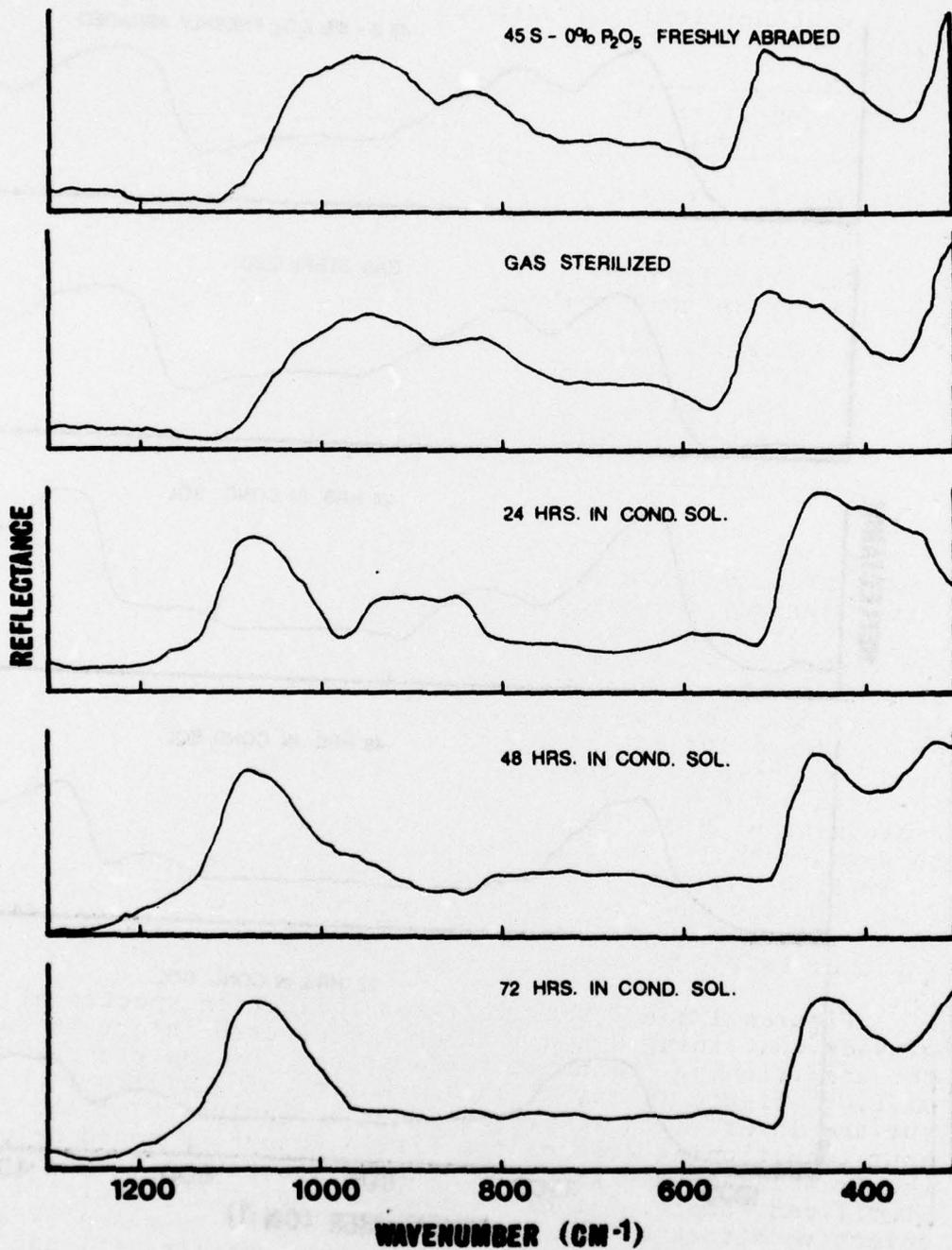
Figure 1. Changes in infrared reflection spectrum of 45S-0% P<sub>2</sub>O<sub>5</sub> glass during conditioning treatment.
