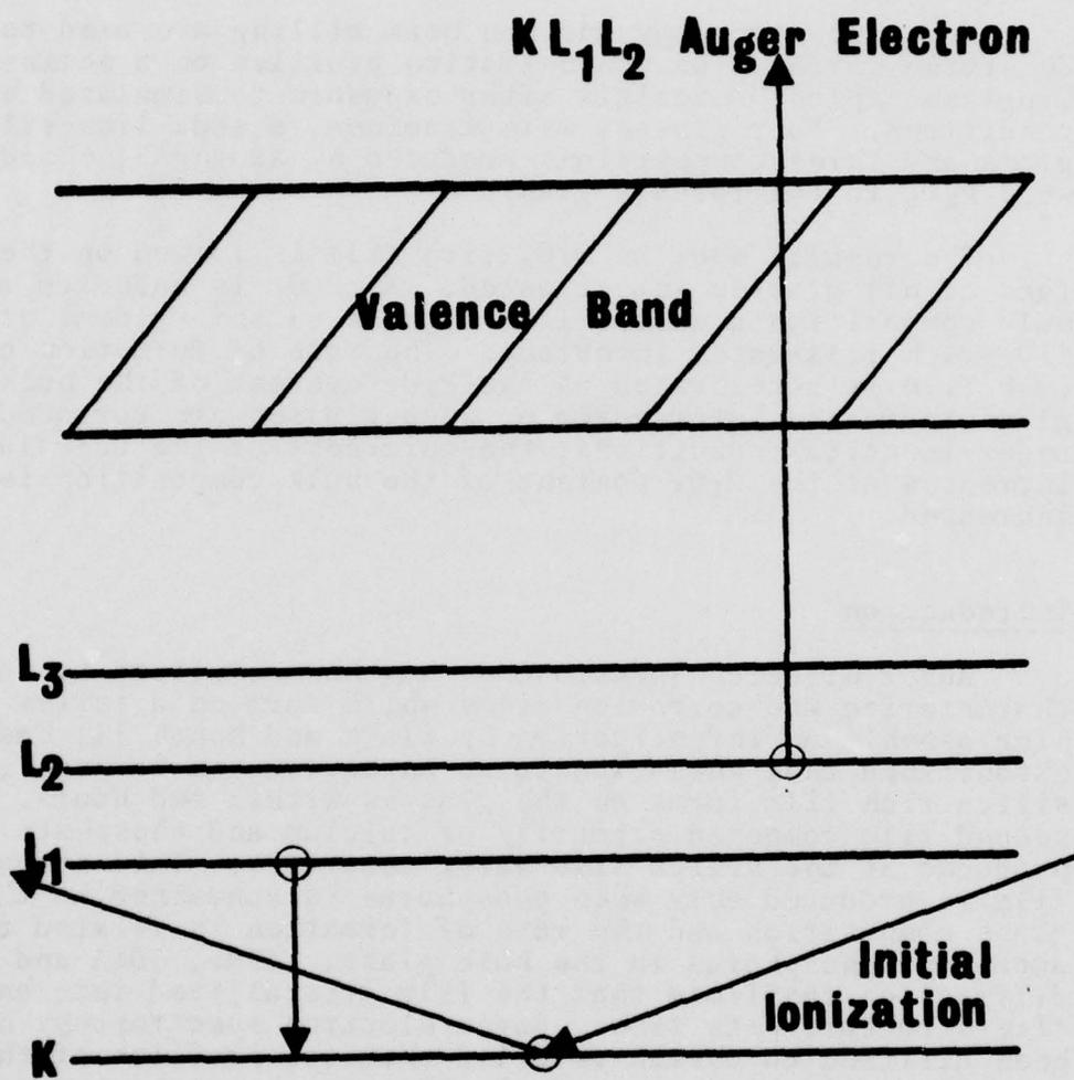
Figure 1. X-ray energy level diagram depicting a  $KL_1L_2$  Auger transition.
