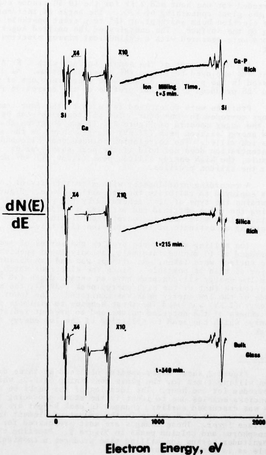
Figure 2. Typical Auger spectra for three depths of ion milling of a 45S-6% P<sub>2</sub>O<sub>5</sub> bioglass corroded one hour at 37°C and pH = 7.4.
