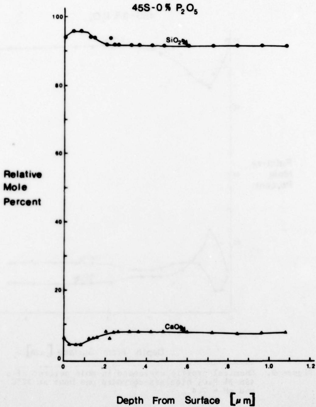
Figure 8. Chemical profile expressed in mole percent of a 45S-0% P<sub>2</sub>O<sub>5</sub> bioglass corroded one hour at 37°C and pH = 7.4.
