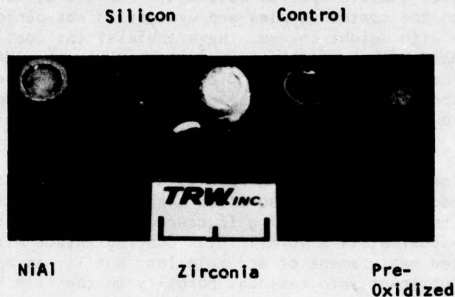
FIGURE 11. Compatibility Test Coupons following 80 Hour Exposure at 1800F. All samples TRW VI A Mod R Base Metal.
