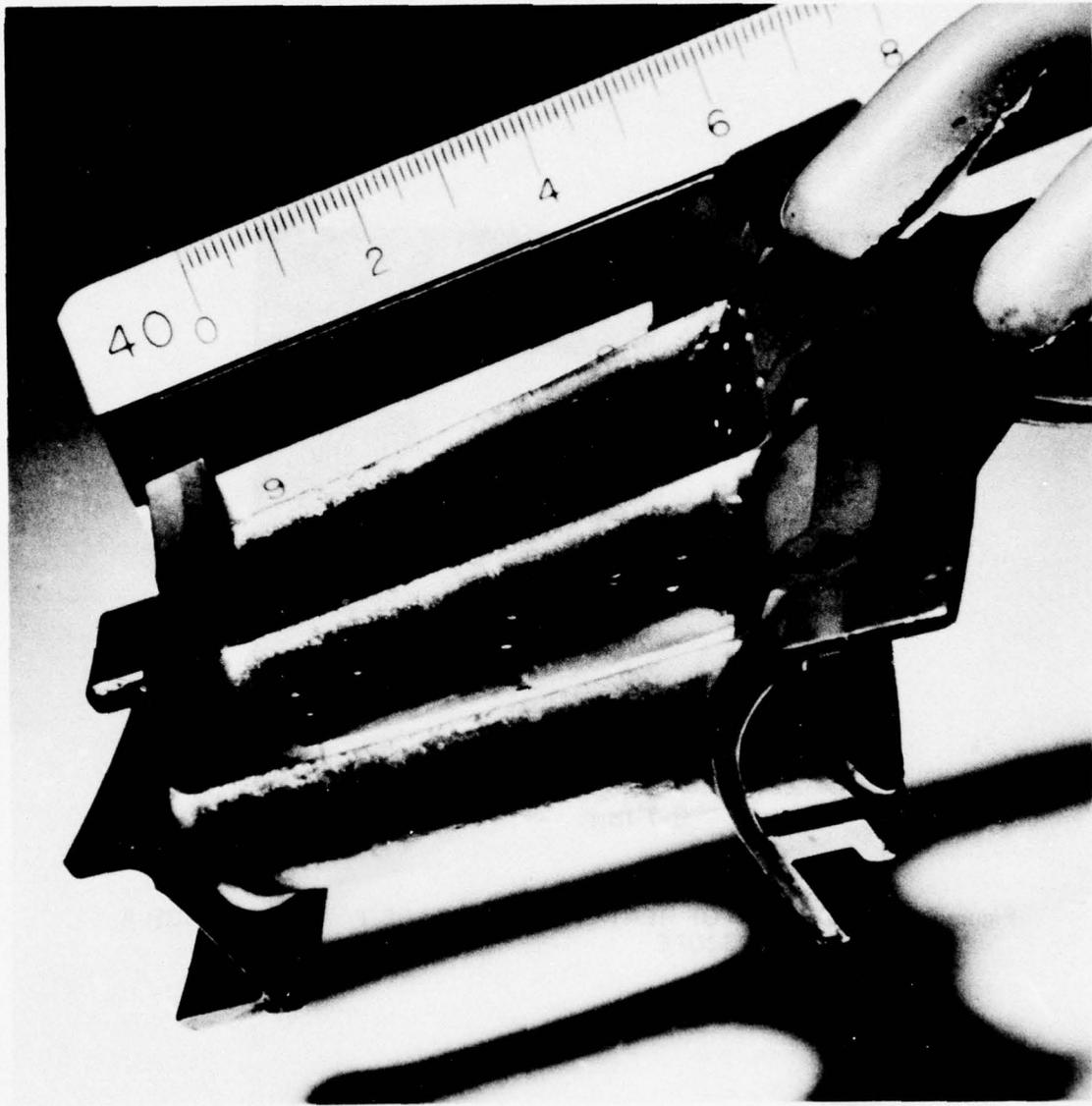
**Figure 6 HOLE LOCATIONS ON AIRFOIL PRESSURE SIDE PRIOR TO INSTALLATION OF HEAT-TRANSFER GAGES**
