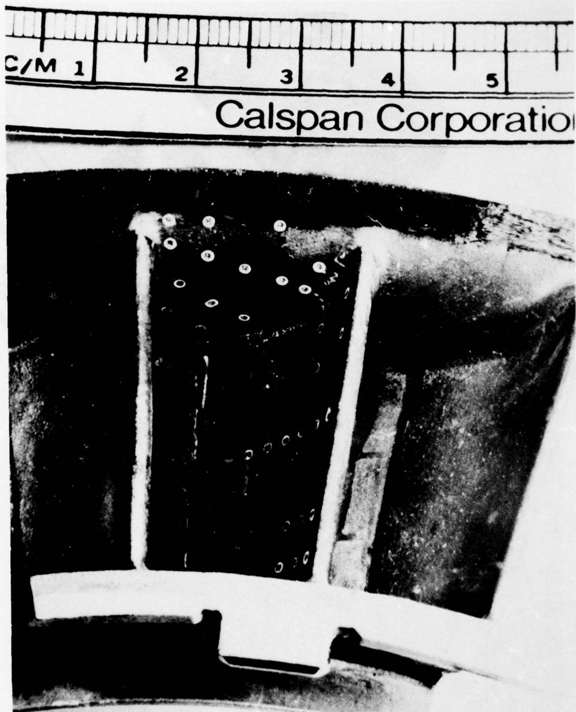
Figure 7 HEAT-TRANSFER GAGES IN TIP ENDWALL AND AIRFOIL PRESSURE SURFACE
