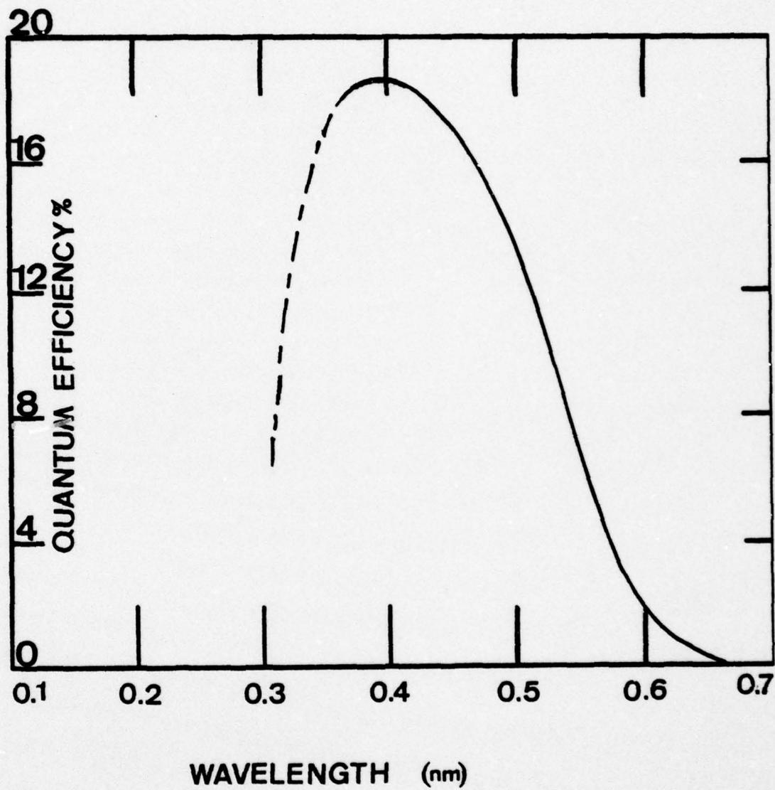
Figure 10. Photomultiplier Tube Spectral Characteristics
