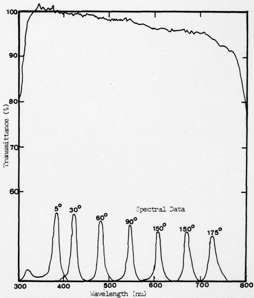
Figure 9. Spectral wedge filter characteristics
