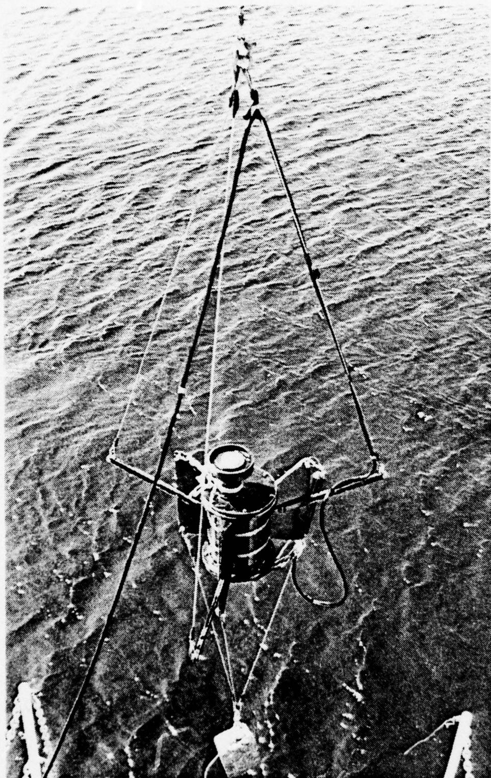
Figure 15. Spectroradiometer Deployment
