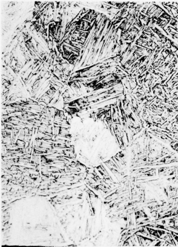
Figure 16. Beta-Transformed Structure in Braces Manufactured in Runs 1 and 2 (250x Mag)
