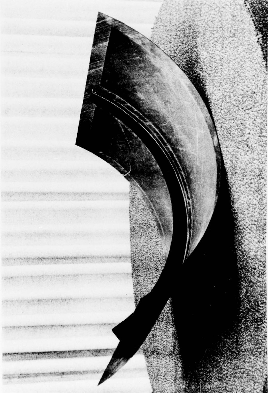
Figure 8-6. Completed Ammunition Bay Door Assembly, Back
