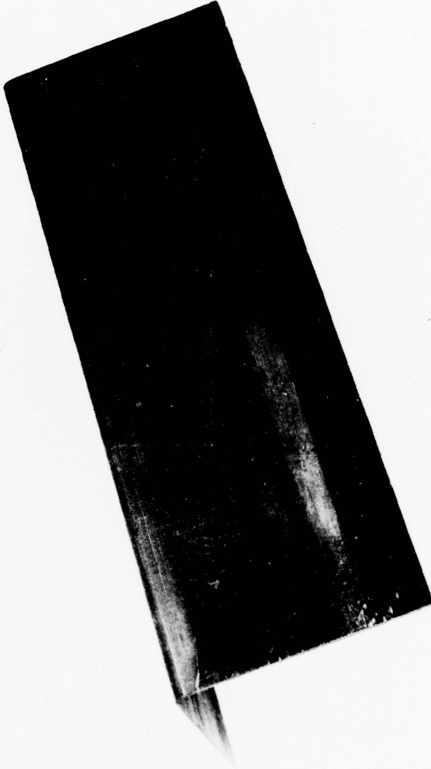
Figure 5-4. Part Formed on Machined Bulk Graphite Tooling
