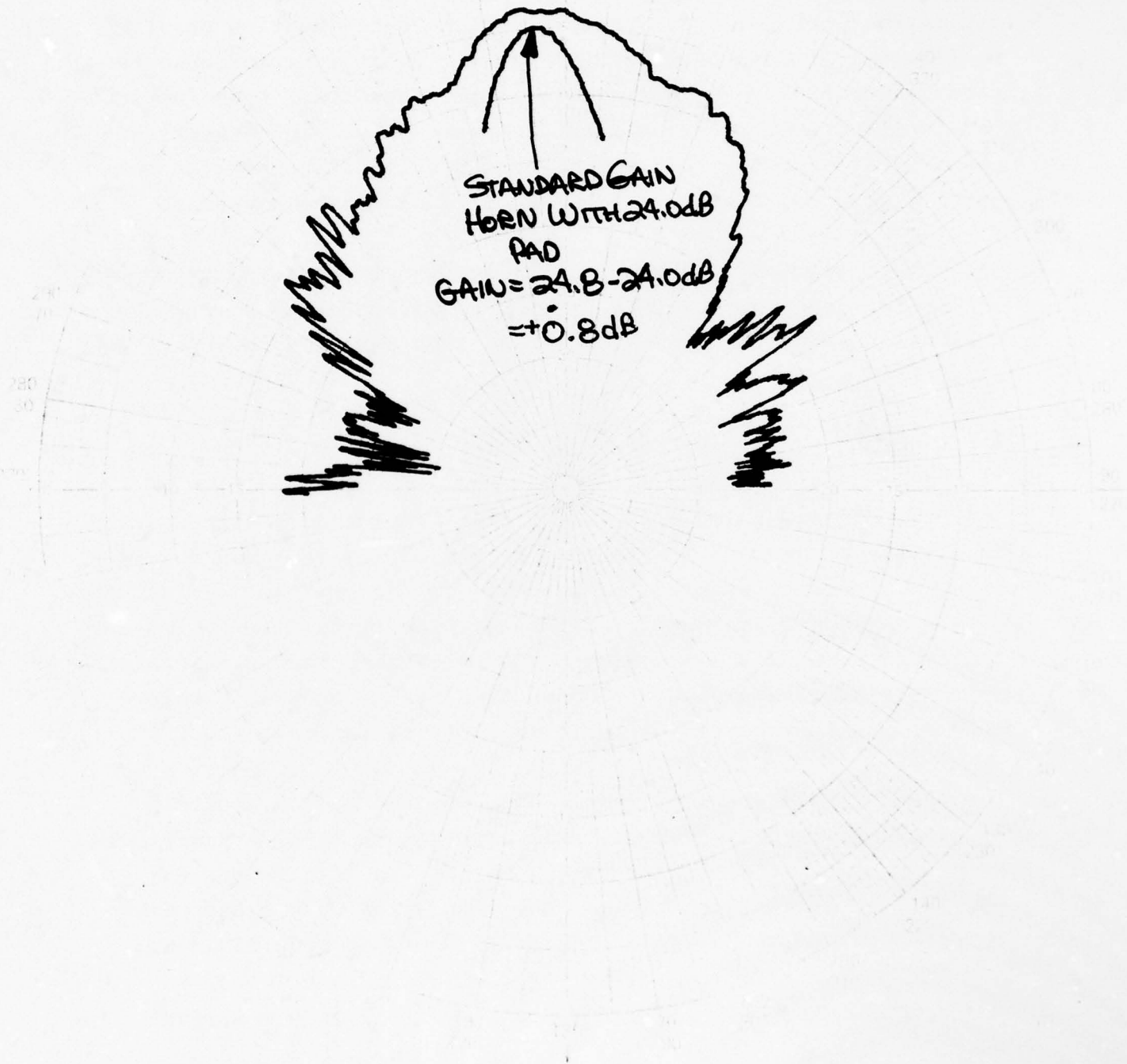
Figure 4-12 H-Plane Radiation Pattern (36.6 GHz) WG Iris Fed
