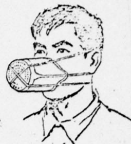
Figure 7-25. Wearable anti-toxic canister.
