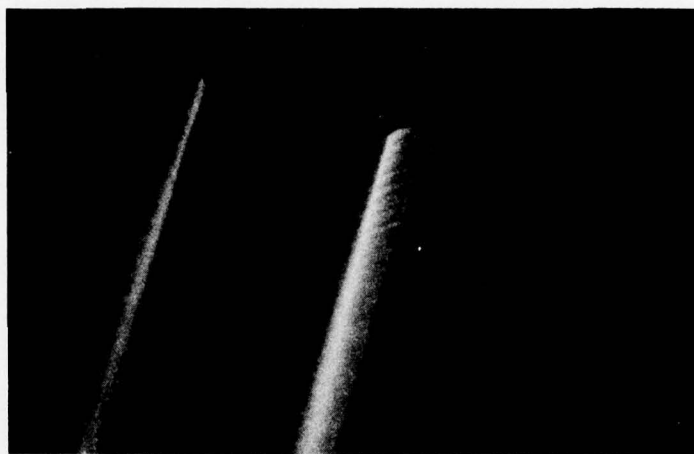
Figure 22. SEM of Plasma Etched Alignment Marker Before Epi
