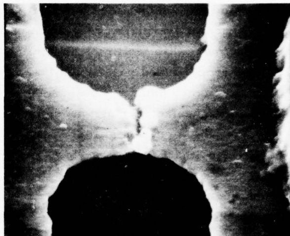
b. Fusing time = 12 ms.
