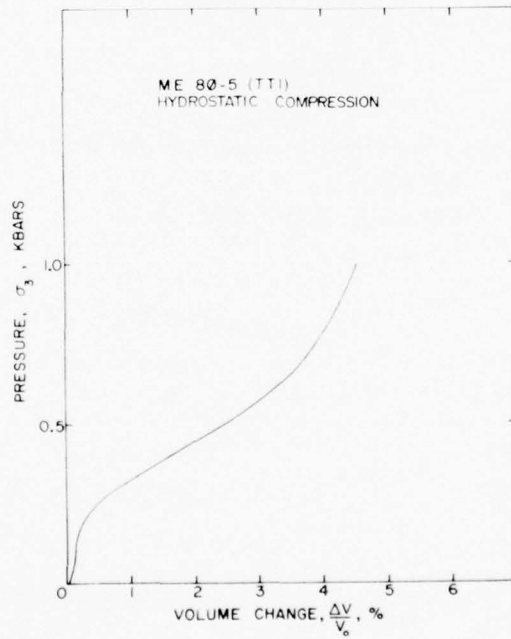
Figure B9. Hydrostatic Compression Results on ME805 Grout Samples (TTI).
