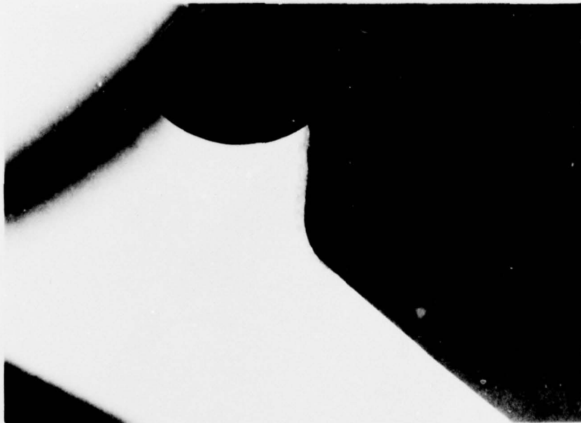
Photo 12. Glime Ice Accumulation on Engine Air Inlet Lip Boot.
