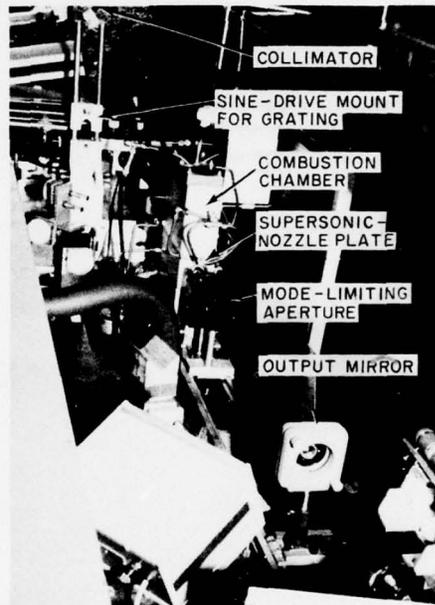
(c) Combustion-driven CW DF laser and laser cavity optics. The sine-drive mount is moved to the left of its normal position for visibility in the photograph.
