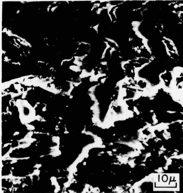
Fig. 4. Galled Surface After Three Revolutions Under Conditions of Fig. 3.
