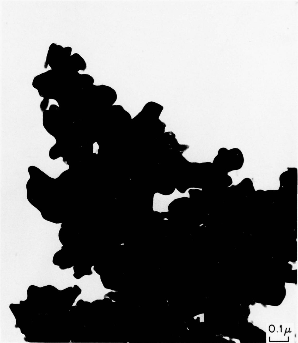
Fig. 4(c) TEM micrograph of a sample of ATA showing layer type structure.
