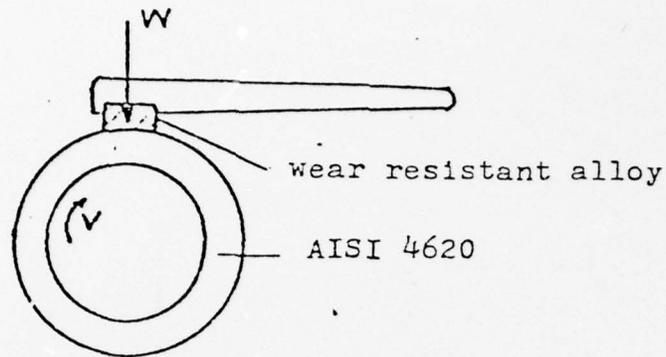
Fig. 2 Dow-Corning Friction and Wear Test Machine.
