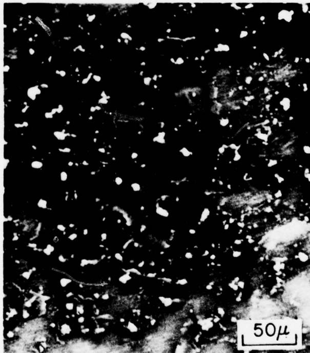
Fig. 8. Plan View Photomicrograph of Surface After 3 Revolutions with  $\text{CCl}_4$  present.
