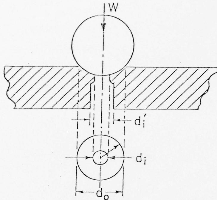
Fig. 2. Area of Contact Between Ball and Impression.
