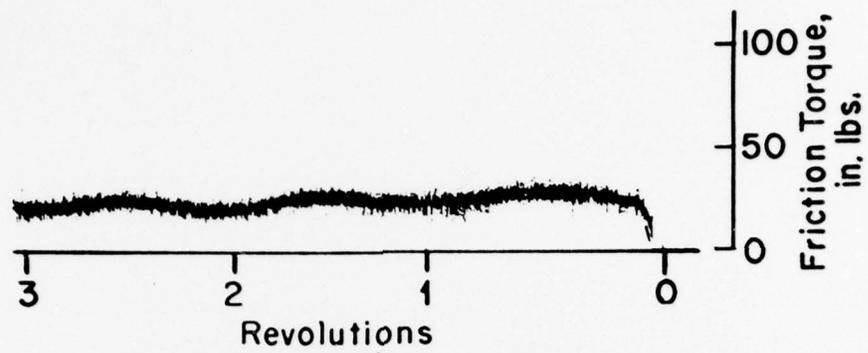
Fig. 7. Friction Torque vs. Rotational Displacement for Sliding with  $\text{CCl}_4$ . Load on sphere = 1000 kg, sliding speed = 2 rpm, hole
