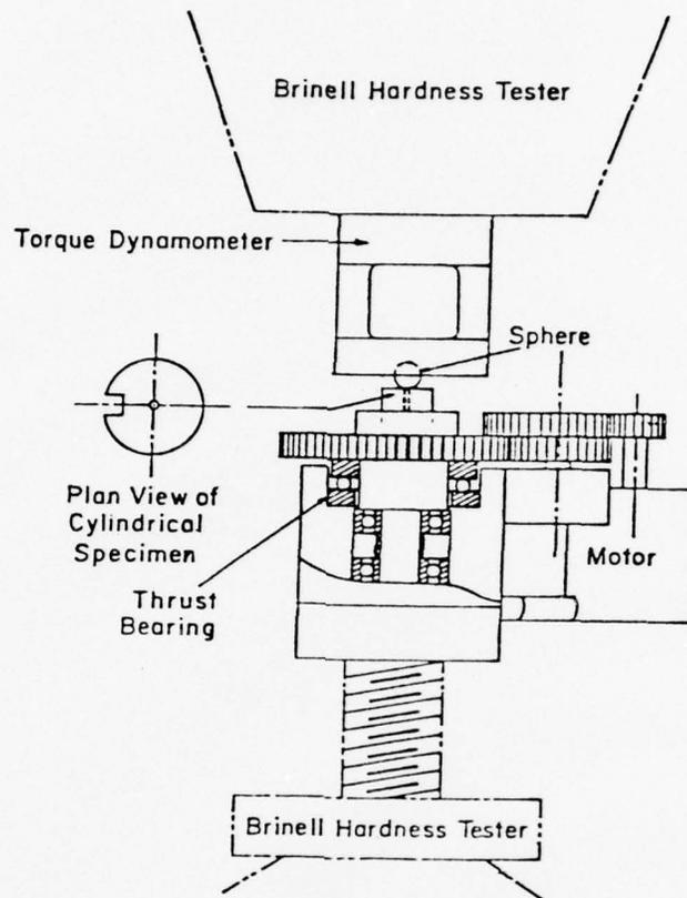
Fig. 1 (a). Schematic Arrangement of Test Apparatus.
