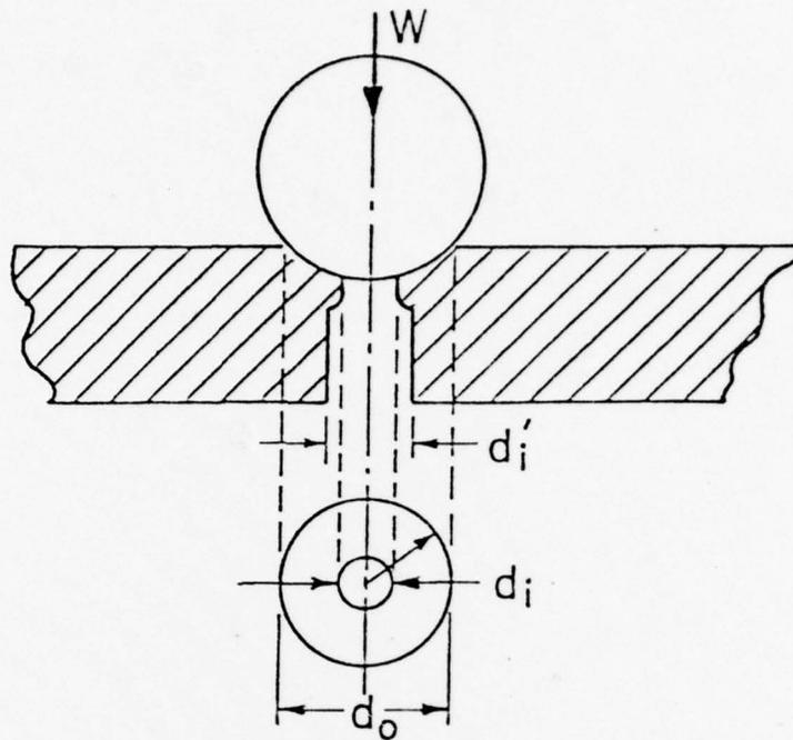
Fig. 1. Principle of Fully Plastic Friction Test.
