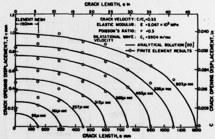
Figure 2. Computed Crack Opening Displacement of a Central Crack Expanding at a Constant Rate in a Uniaxial Stress Field of 68.9 MPa (10,000 psi).
