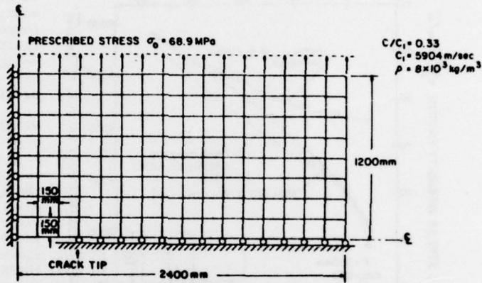
Figure 1. Finite Element Breakdown for Broberg's Problem.
