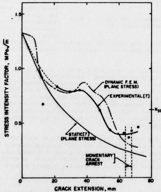
Figure 7. Stress Intensity Factors in a Wedge-Loaded DCB Specimen [7]
