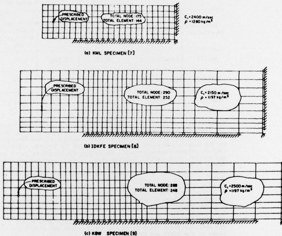
Figure 5. Finite Element Breakdowns of Three DCB Specimens
