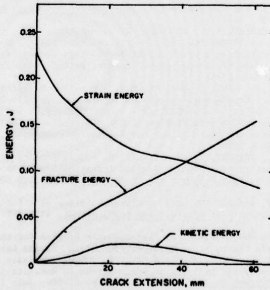
Figure 10. Energies in a Wedge-Loaded DCB Specimen [9].
